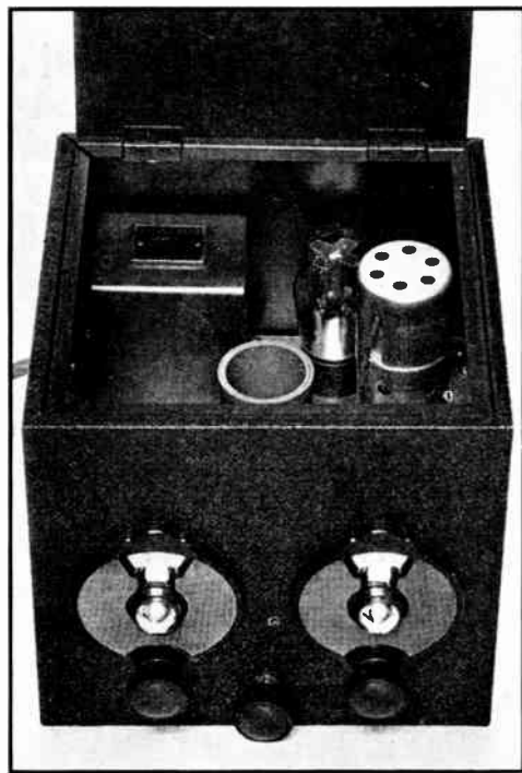
FIG. 512 — THIS TWO-TUBE RECEIVER HAS A CONTINUOUS FREQUENCY RANGE OF 1450 TO 41,000 KILOCYCLES AND GIVES COMPLETE BAND-SPREAD ON FIVE AMATEUR BANDS
