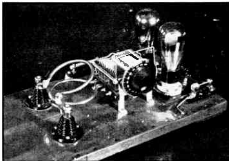
FIG. 902 — A 56-MC. EXPERIMENTAL OSCILLATOR The various components can be located by reference to the circuit of Fig. 901. The antenna coil is a half turn mounted over the plate coil.
