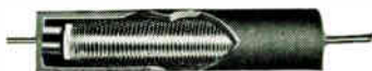
Cross Section — showing progressive interleaved windings for higher resistance values in less space.
