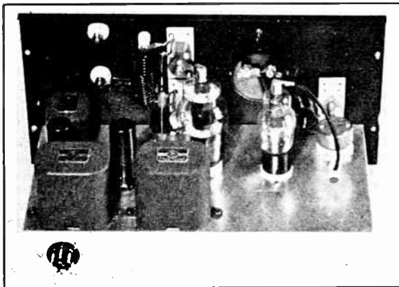
Fig. 2813 — The 89 at the right doubles from a 20-meter crystal, driving the 807 as a doubler on five or straight through on ten. The 6J5-6N7 Class-B modulator at the left provides plenty of push from a carbon mike, even with 30 watts into the 807. (W2JCR, August, 1939, QST.)
