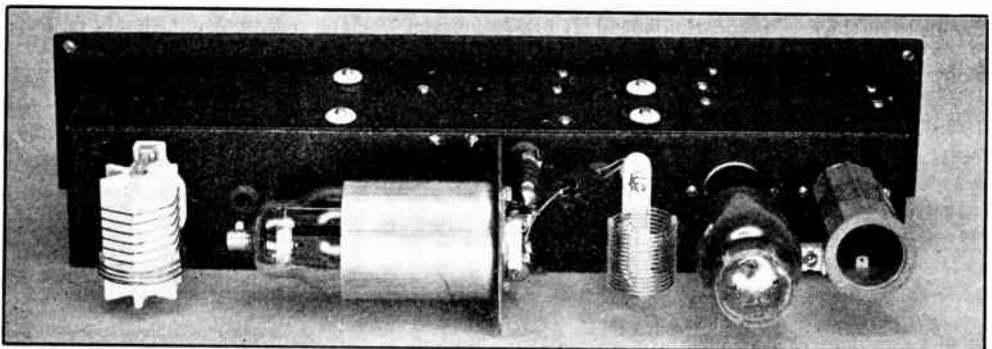
Fig. 1017 — The 4-prong socket for the cathode coil, the octal for the 6L6 oscillator and the 5-prong socket for the Coto coils used in the output tank circuit are sub-mounted in the rear edge of the chassis. The mounting for the National AR coils used in the oscillator plate circuit is fastened on short cone insulators, while the socket for the 807 is sub-mounted in the small steel partition. The grid r.f. choke and screen and cathode by-pass
