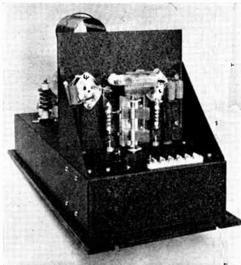
Fig. 1035 — The grid-circuit components of the 450-watt amplifier are mounted on this side of the partition which is braced by standard 5-in. triangular brackets. The tank condenser is mounted by means of a screw in the hole which remains when the shield between the stators is removed. The ceramic terminal strip is for all external connections except for positive high voltage for which a special safety terminal is provided. A large clearance hole should be cut in the chassis for the condenser shaft. The shaft should come at the center line of the chassis.
