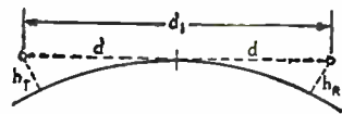
Fig. 907 — Method of determining total line-of-sight distance when both transmitter and receiver are elevated. Since only earth curvature is taken into account in Fig. 906, irregularities in the ground between the transmitting and receiving points must be considered for each actual path.
