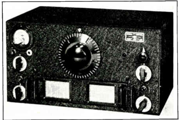
Fig. 1111—The National HRO 9-tube superheterodyne. The gang of four coils is plugged in under the tuning dial.
