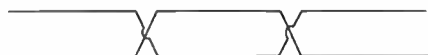
Fig. 1008 — Method of transposing a two-wire open transmission line to preserve balance to ground and nearby objects.
