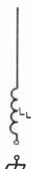
Fig. 19-31 — The capacitive reactance at frequencies lower than the resonant frequency of the whip can be canceled out by adding an equivalent inductive reactance in the form of a loading coil in series with the antenna.
