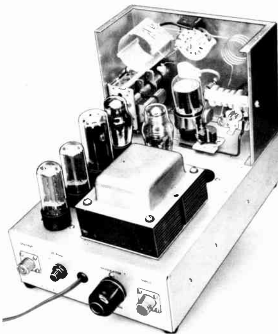
Fig. 6-49—Rear view of the 90-watt all-purpose amplifier with the cane-metal cover removed. One voltage-regulator tube has been removed from its socket (right edge of transformer) to allow the neutralizing capacitor and plate blocking capacitor to be seen. The plate r.f. choke ( RFC_3 in Fig. 6-50) is mounted on one side wall, and the load capacitor and safety choke ( C_4 and RFC_4 in Fig. 6-50) are mounted on the far side wall.
