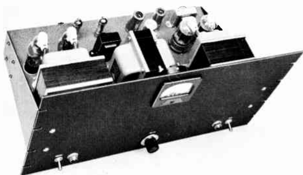
Fig. 9-23—Class-AB 1 modulator using 6146s, complete with speech amplifier and power supply. The relay-rack panel is 10½-inches high. Plate- and filament-supply primary switches, each with its own pilot lamp, are near the lower edge of the panel. The gain control is at lower center. Along the front of the chassis, just behind the panel, are the plate power transformer, filter choke, and modulation transformer, going from left to right. The tubes at the left are the 816 rectifiers, with the 6146s at the right. Along the rear edge are the two voltage-regulator tubes, the 12AX7 and 6C4 speech amplifier tubes, and the inter-stage audio transformer, T_1 .
