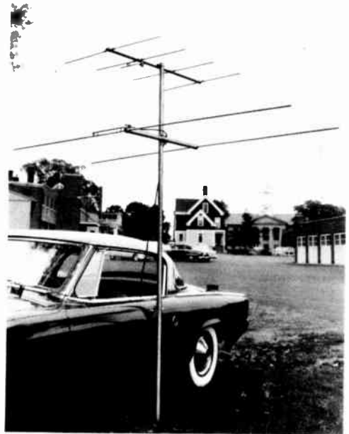
Fig. 18-5—Two-element 50-Mc. and four-element 144-Mc. arrays designed for portable use. Support is sectional TV masting clamped to car door handle. Elements of 50-Mc. array are made in three sections, for stowing in back of car. Antenna for 144 Mc. is cut-down TV array. Both use gamma match, as shown in Fig. 18-6.
