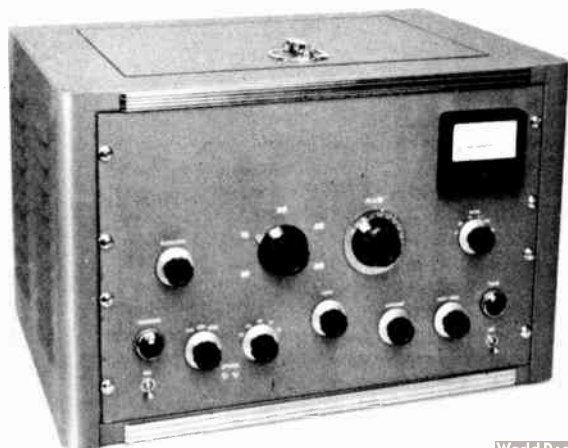
Fig. 6-58—A 500-watt transmitter. Power supplies and a differential keyer are included. It operates with the external v.f.o. tuner shown in Fig. 6-59. Controls along the bottom, from left to right, are for low-voltage power, v.f.o./crystals/s.s.b. switch, driver tank switch, driver tank capacitor, final loading, v.f.o. set switch, and high-voltage. Above, from left to right, are controls for excitation, final tank switch, final tank capacitor and meter switch. The band-switch pointer is made by cutting down the metal skirt of a dial similar to the one to the right.
