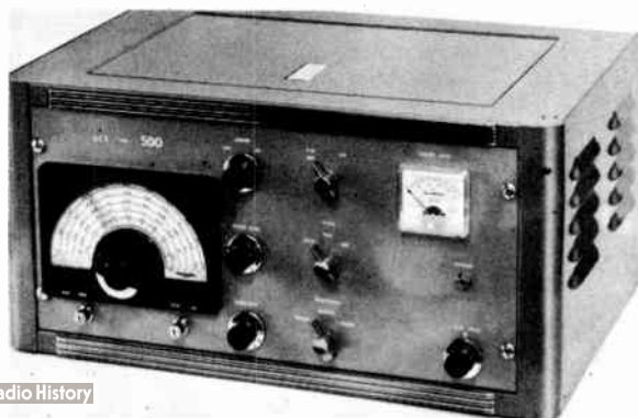
Fig. 5-51—The DCS-500 double-conversion superheterodyne. Left bottom, antenna trimmer, 100-kc. calibrator switch; center, left, top to bottom, noise-limiter switch, volume control, sensitivity control; center, right, b.f.o. switch, a.g.c. speed, selectivity; right, headphone jack, b.f.o. pitch control. The dial is a National ICN. Front panel is 8½ inches high; the receiver is mounted in a Bud CR-1741 rack cabinet.
