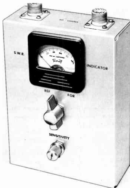
Fig. 21-42—The Monimatch, an s.w.r. monitor that can be left in the line at all times. The unit shown here will handle a kilowatt.
