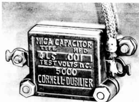
Fig. 23-10—Bypassing with a mica capacitor the end of a high-voltage lead. The end of the shield braid is soldered to a lug fastened to the chassis directly underneath. The other terminal of the capacitor is similarly bolted directly to the chassis. When the bypass is used at a terminal connection block the "hot" lead should be soldered directly to the terminal, if possible, but in any event connected to it by a very short lead.
