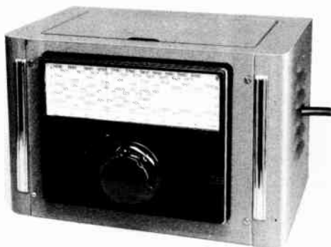
Fig. 6-62—The remote v.f.o. tuning unit is housed in a standard metal cabinet. The cable at the right plugs into the main chassis.
