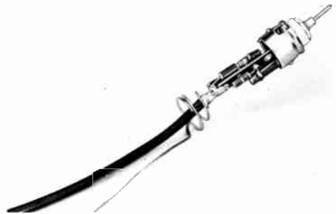
Fig. 21-31—Close-up of the inside of the probe. The 1N34A crystal diode rectifier, calibrating resistor, and input capacitor are mounted tight to the terminal strip with shortest leads possible. Spaghetti tubing is placed on the diode leads to prevent accidental short circuits. The tube-shield spring and REXIBLE-copper grounding lead are soldered to the cable braid (the cable is RG-58/U coax). The tip can be either a phone tip or a short pointed piece of heavy wire.
