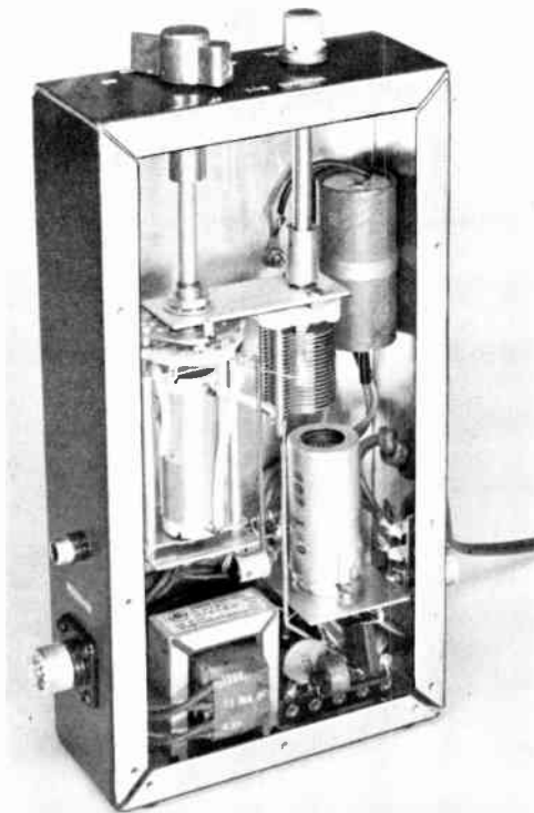
Fig. 8-16—The electronic t.r. switch is built in a 5 X 9 X 2 1/2-inch chassis; the bottom plate has been removed to show the placement of parts. Although two receiver outlets are shown on the near face (a phono jack and a coaxial receptacle), only one is required, depending upon one's choice of cable termination.
