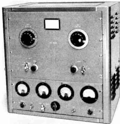
Fig. 6-68—The kilowatt 4-400A amplifier and its control unit are mounted in a 21-inch gray hammer-tone rack cabinet (Bud CR-1727). Shelf brackets (Bud SA-1350) are mounted on both sides of the cabinet to hold the amplifier chassis. Below the meters, from left to right: filament pilot light, key-type a.c. switch, Class AB 1 /C bias switch, screen autotransformer, plate switch and plate pilot light.
