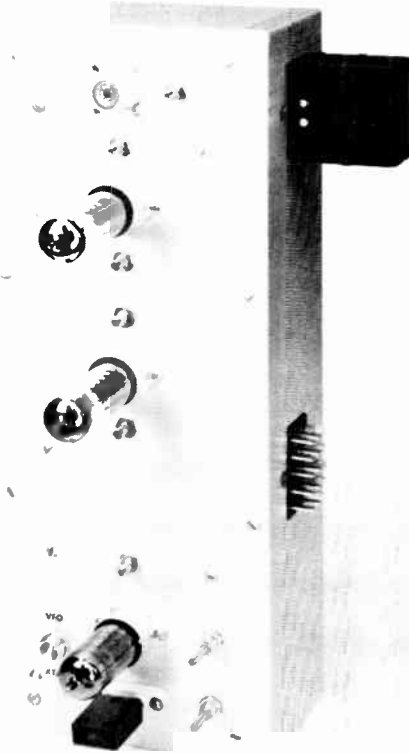
Fig. 17-5—Top view of the 144-Mc. transmitter/driver. The power socket (upper right) with jumper plug in place, is used with the 432-Mc. tripler amplifier.
