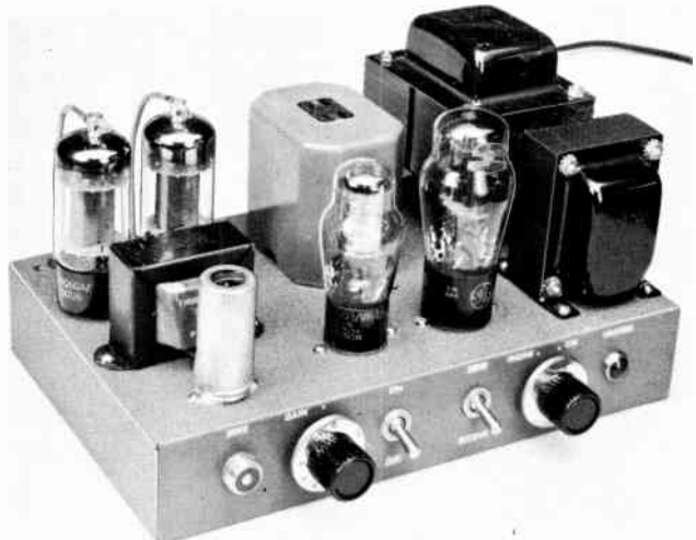
Fig. 9-17—A modulator for transmitters operating at plate inputs up to 50 watts. The speech amplifier and modulator are on the left in this view; power supply components are on the right. The chassis is 7 × 11 × 2 inches.
