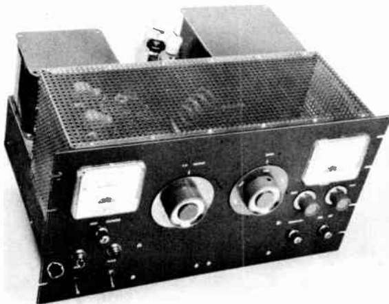
Fig. 6-64—This amplifier operates at a plate input of approximately 500 watts, uses a pair of 811As in grounded-grid, and is complete with power supply on a 13 \times 17 \times 4 -inch chassis. The rack panel is 10\frac{1}{2} \times 19 inches. Front-panel controls include the plate tuning capacitor and band switch in the center, filament and plate power switches with their pilot lights at the lower left, sensitivity control and forward-reflected power switch for the directional coupler at the lower right, variable loading capacitor and auxiliary loading-capacitor switch underneath the 0.1 milliammeter at the right, and the grid-cathode milliammeter with its switch at the upper left. The filter choke, 866As and plate transformer occupy the rear section of the chassis.
