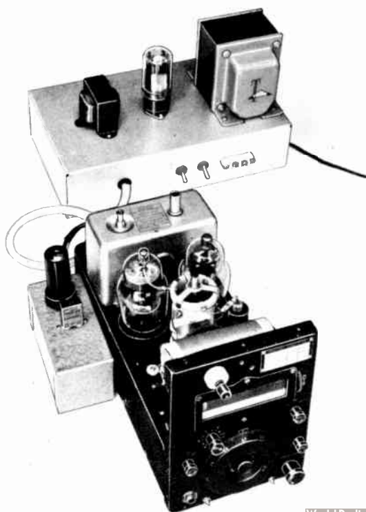
Fig. 6-89—The complete Novice setup, in this case using the 80-meter (BC-696) transmitter. Note the key jack at the lower-left corner of the transmitter panel. The crystal oscillator is connected to the transmitter oscillator-tube socket with a short length of cable terminating in an octal plug. A small notch should be cut in the transmitter cover to provide clearance for the cable when the cover is installed.
