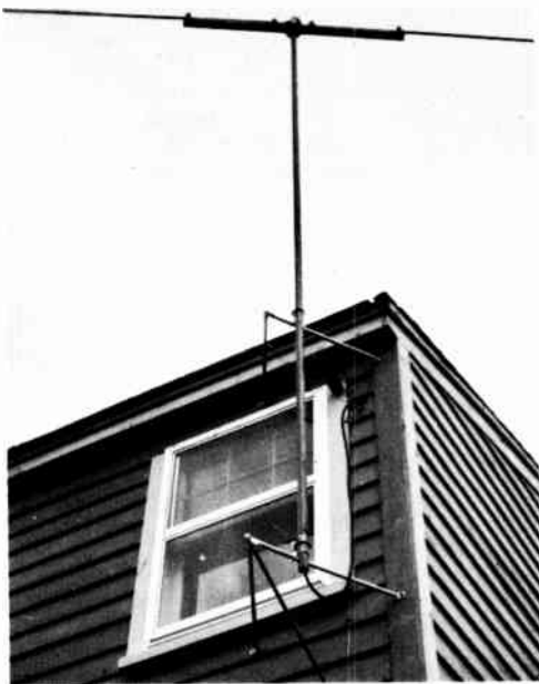
Fig. 14-61—Over-all view of the antenna and mounting. The feedline comes out of the bottom of the mast and through the wall into the shack.
