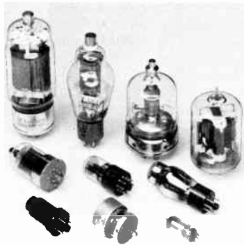
Representative tube types. Transmitting tubes having up to 500-watt capability are shown in the back row. The tube with the top cap in the middle row is a low-power transmitting type. Others are receiving tubes, with the exception of the one in the center foreground which is a v.h.f. transmitting type.
