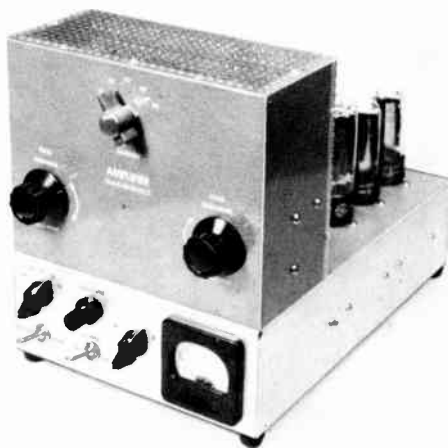
Fig. 6-48—Front view of the 6146 all-purpose amplifier. The upper panel is part of an 8 × 6 × 3½-inch Minibox (Bud CU-2109); the ventilated shielding of Reynolds Aluminium cane metal is fastened to the Minibox and base with sheet-metal screws.
