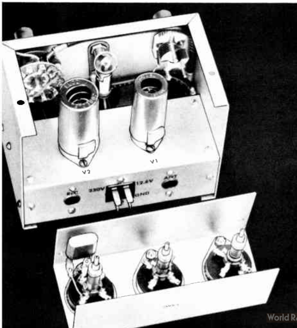
Fig. 19-7—Homemade L-shaped chassis, mounted on small brackets fastened to the side walls of the converter housing, is 4\frac{1}{8} inches long, 2 inches wide and 1\frac{1}{2} inches deep. V_1 is mounted on the chassis to the right of V_2 as seen in this rear view. J_1 , J_3 and J_2 are in line in that order from right to left across the rear wall of the chassis. An interior view of a coil compartment is shown in the foreground. Terminals of the coils are soldered directly to the socket terminals. Notice that the crystal for the oscillator is mounted adjacent to L_4 .
