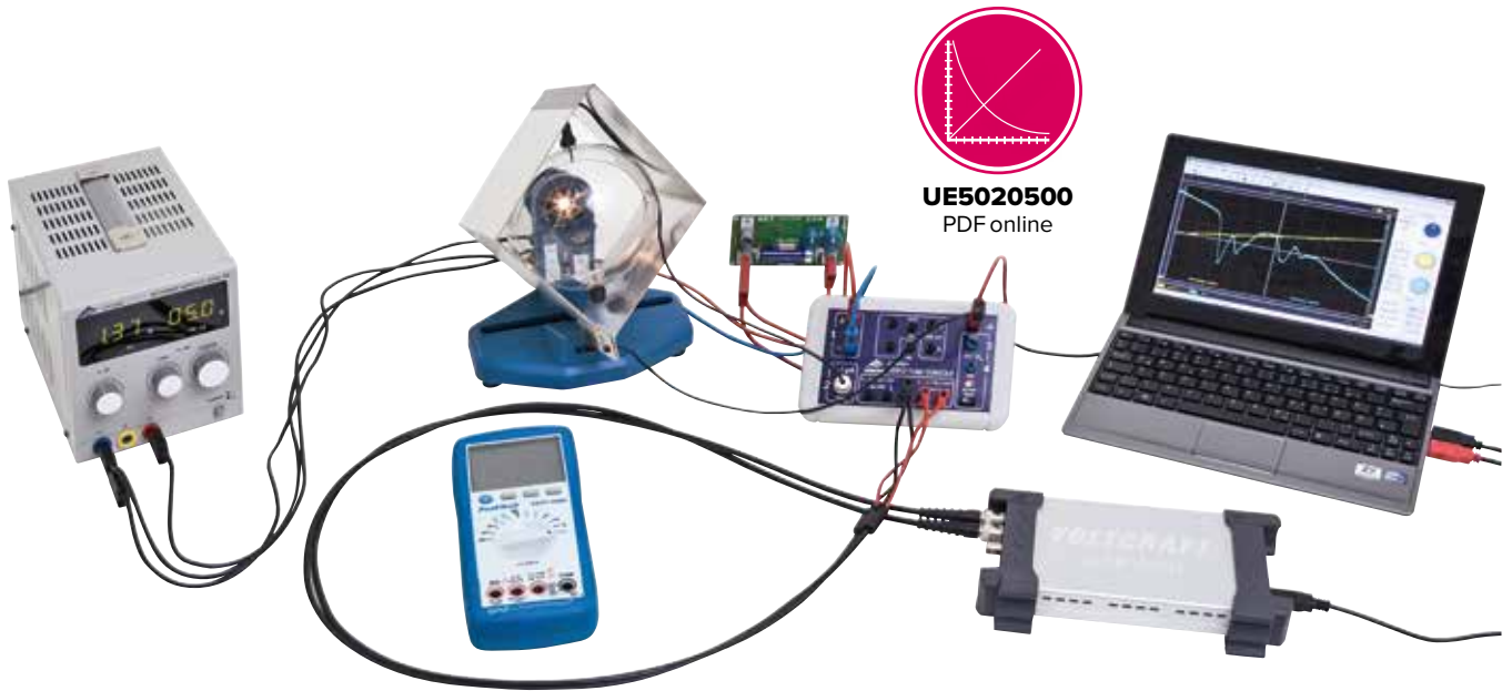
Experiment set-up with the control unit for critical potentials tubes
