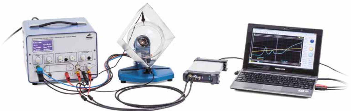
Experiment set-up with the control unit for the Franck-Hertz experiment
