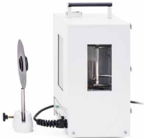
Experiment set-up for transmissive illumination of sodium fluorescence tube with a beam of white light
