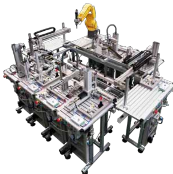
Configuration of 10 stations with transfer
