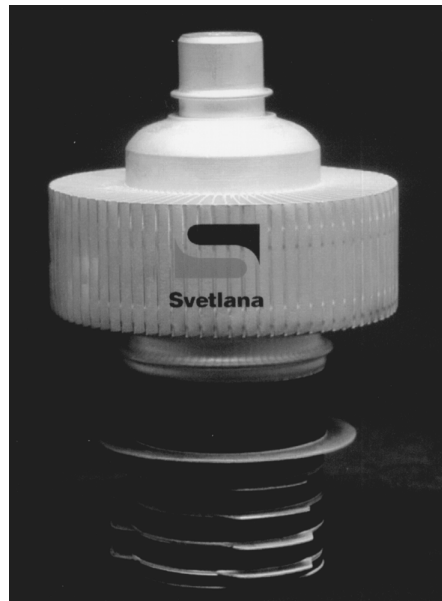
FIGURE 3.14 5CX1500B power pentode device. (Courtesy of Svetlana Electron Devices, Huntsville, AL.)
