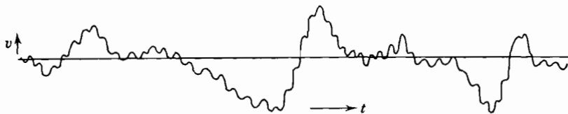
FIG. 15.4. Random noise passed through a low-pass filter.
