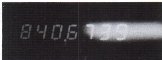
Figure 14. Effect of anti-reflection surface on an optical filter.
