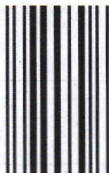
BAR WIDTH 0.3 mm (0.012 in.) BLACK & WHITE R WHITE > 75%, PCS > 0.9 KODAGRAPH TRANSTAR TC5® PAPER
