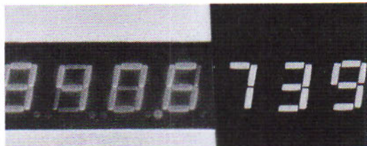
Figure 1. Effect of wavelength optical filter on LED display.
