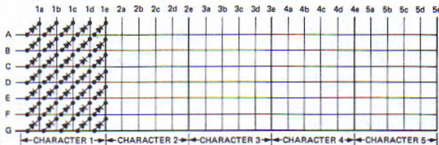
5082-7100/7101/7102 Schematic Wiring Diagram
