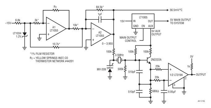
Figure 6. Temperature Compensated Crystal Oscillator (TXCO)
