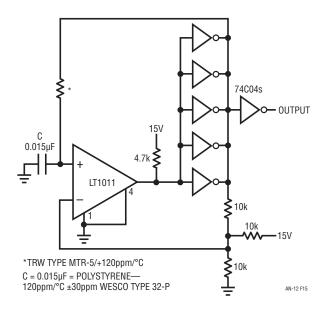
Figure 15. Stable RC Oscillator
