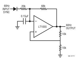
Figure 11. Synchronized Oscillator
