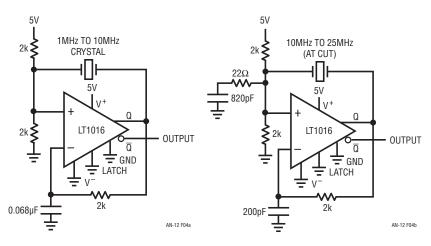
Figure 4a. 1MHz to 10MHz Crystal Oscillator
