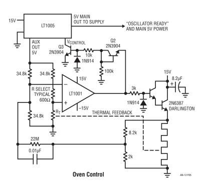
Figure 5. Ovenized Oscillator
