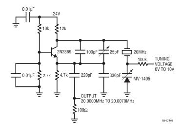
Figure 8. Voltage Controlled Crystal Oscillator (VCXO)
