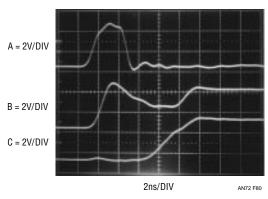
Figure 80. Results of Disconnecting C<sub>T</sub>-Originated Feedforward Path. Output (Trace B) Sags for 8ns Before C1 (Trace C) Can Restore Its Amplitude
