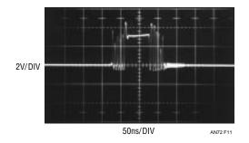
Figure 11. 3pF Stray Capacitive Feedback with 3k  $\Omega$  Source Can Cause Oscillation
