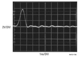
Figure 26. The Test Pulse Appears Smaller and Slower on a 350MHz Instrument ( $t_{RISE}$  = 1ns). Deliberate Poor Grounding Creates Rippling After the Pulse Falls. Direct 50 $\Omega$  Connection Is Used
