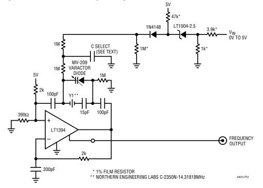
Figure 51. A  $4\times$  NTSC Sub-Carrier Voltage-Tunable Crystal Oscillator. Tuning Range and Bandwidth Accommodate Variety of Phase Locked Loops
