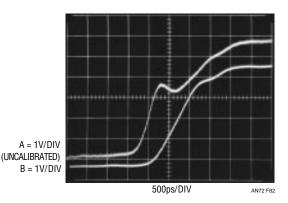
Figure 82. Pulse Stretcher Waveforms in 3.9GHz Bandpass Show 650ps Output Rise and Delay Times (Trace B). Nonlinear Loading Causes Input Transition Aberration (Trace A), but Is Not Deleterious. Trace Granularity Derives from Sampling Oscilloscope Operation
