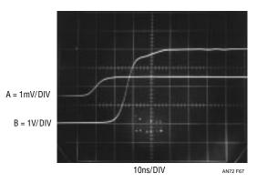
Figure 67. Parallel Path Comparator Shows 18ns Response (Trace B) to 500µV Overdrive (Trace A)
