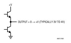
Figure A1. Simplified LT1394 Output Stage
