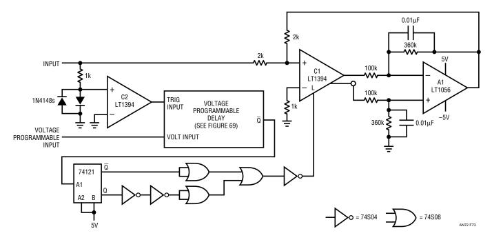
Figure 73. 10ns Sample-and-Hold for Repetitive Signals. Feedback Loop Around Comparator and Programmable Delay Allow Controllable Sampling of Input
