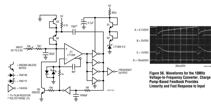
Figure 55. Simple Charge Pump-Based 10MHz Voltage-to-Frequency Converter Has 40dB Dynamic Range, Operates from 5V Supply
