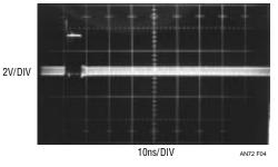
Figure 4. LT1394 Response with Poor Bypassing
