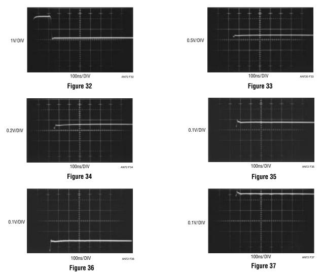
Figures 32 to 37: The Overdrive Limit Is Determined by Progressively Increasing Oscilloscope Gain and Watching for Waveform Aberrations
