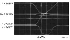
Figure 71. High Speed Expansion of Figure 70. Ramp (Trace B) Begins When Trigger (Trace A) Falls and Current Source Turns On (Trace C). Trace D is Output
