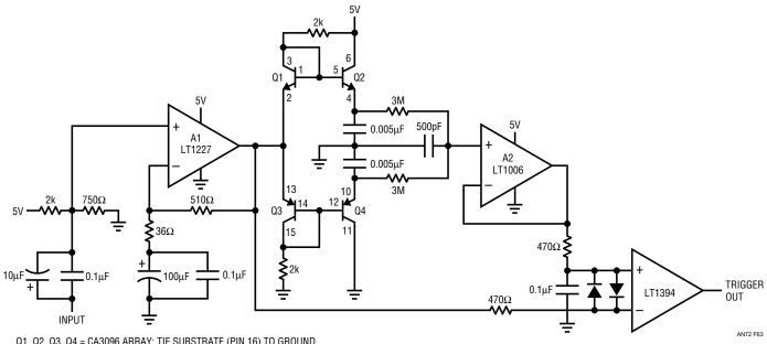
01, 02, 03, 04 = CA3096 ARRAY: TIE SUBSTRATE (PIN 16) TO GROUND = 1N4148
