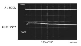
Figure 43. Response of  $10\mu F$  Aluminum Capacitor
