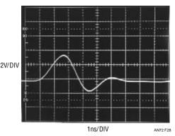
Figure 28. Test Pulse Measures Only 3V High on a 250MHz 'Scope with Significant Waveform Distortion. 290MHz 10 $\times$  Probe Used
