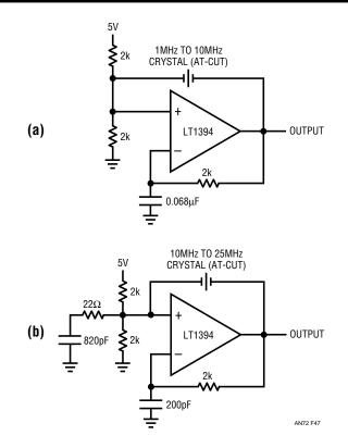
Figure 47. Crystal Oscillators for Outputs to 30MHz. Circuit (b)'s Damper Network Supresses Overtone Crystal's Harmonic Modes
