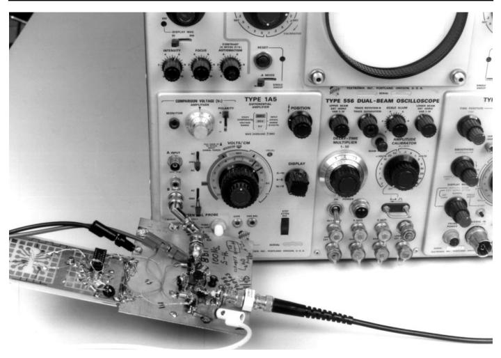
Figure 18. Sometimes the Best Probe Is No Probe. Direct Connection to the Oscilloscope Eliminates a  $10 \times$  Probe's Attenuation and Possible Grounding Problems
