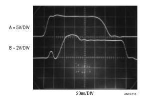
Figure 15. Input Common Mode Overdrive Generates Odd Outputs
