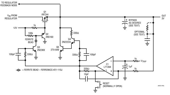
Figure 83. A 20ns Response Time Overvoltage Protection Circuit. Latching Comparator Drives a Turn-Off Optimized Series — Shunt Switch
