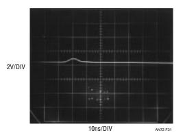
Figure 31. A 50MHz Instrument Barely Grunts. 10V, 350ps Test Pulse Measures Only 0.5V High with 7ns Rise and Fall Times!
