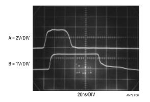
Figure 8. Overdriven FET Probe Causes Delayed, Tailing Response
