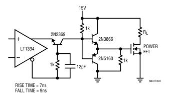
Figure A4. Noninverting Voltage Gain Level Shift
