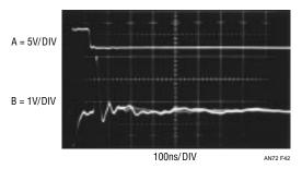
Figure 42. Response of Unbypassed Line
