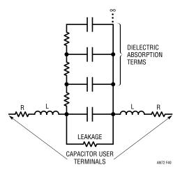
Figure 40. Parasitic Terms of a Capacitor
