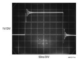
Figure 14. Lengthy, Unterminated Output Lines Ring from Reflections
