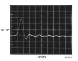
Figure 27. Test Pulse on the Same 350MHz Oscilloscope Using a 3GHz 10  $\times$  Probe. Deliberate Poor Grounding Maintains Rippling Residue
