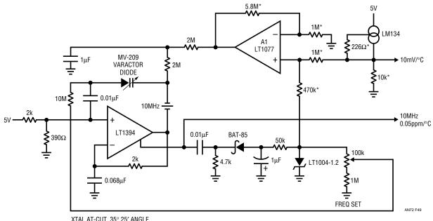
XTAL AT-CUT, 35° 25′ ANGLE \* 1% FILM RESISTOR
