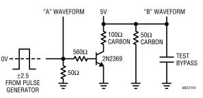
Figure 41. Bypass Capacitor Test Circuit
