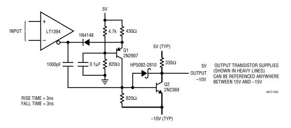
Figure A3. Level Shift with Inverting Voltage Gain—Bipolar Swing
