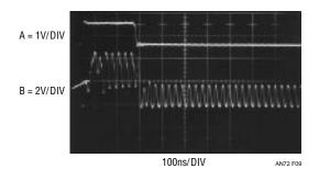
Figure 9. Excessive LT1394 Ground Path Resistance Causes Oscillation
