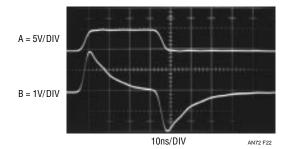
Figure 22. Test Circuit Output with 9pF Probe and 1/4-Inch Ground Strap
