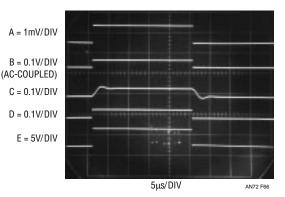
Figure 66. 500  $\mu$ V Input (Trace A) Is Split into Wideband and Low Frequency Gain Paths (Traces B and C) and Recombined (Trace D). Comparator Output Is Trace E
