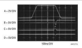
Figure 74. Sampling Pulse (Trace D) May Be Positioned at Desired Point on Input Waveform (Trace A)
