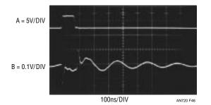
Figure 46. Some Paralleled Combinations Can Ring. Try Before Specifying!
