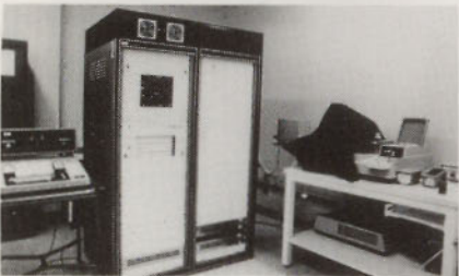
Finished wafers are tested on Litronix designed and built micro processor controlled automatic testers.
