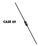
Subminiature silicon rectifier with glass passivated surface in void-free, flame-proof, silicone polymer case. Tested in accordance with MIL-S-19500/228 for military applications requiring up to 1 ampere output at  $100^{\circ}$ C.
