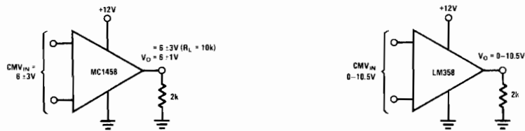
FIGURE 1. Worst Case Signal Levels with +12V Supply
