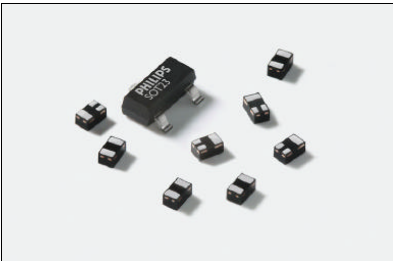
SOT88x compared to SOT23
