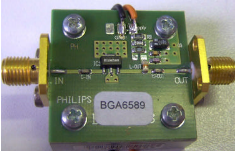
The Demo Board with medium power wide-band gainblock BGA6589. (See also the objective datasheet BGA6589)
