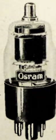
The Osram Z62 is an indirectly heated pentode with a high slope and designed for use in short-wave receivers or wide-band amplifiers. The short seal gives improved performance up to 60 Mc.
