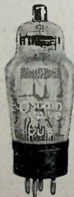
A mercury-vapour rectifier of the GU50 class. These rectifiers are half-wave types, and are used extensively in amateur and commercial power supply equipments. When in operation they exhibit a blue glow. The filament must always be switched on for about 30 seconds before the anode voltage is applied.
