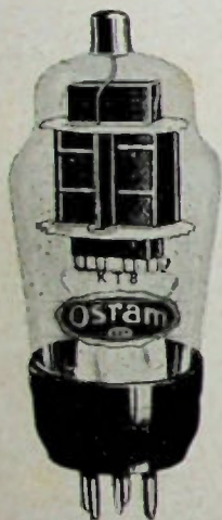
The Osram KT8 is a screen radio frequency transmitting tetrode rated at 25 watts anode dissipation. The valve has an indirectly heated cathode aligned grids and beam confining plates.
