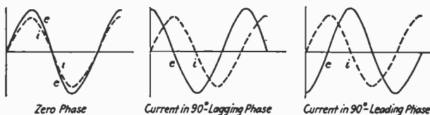
FIG. 2.—Phase in a-c circuits.
