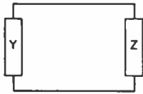
FIG. 9. Resonant circuit consisting of dual elements.
