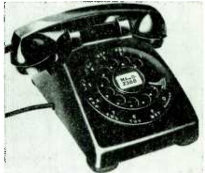
FIG. 3. Typical dial telephone set, 500 type.
