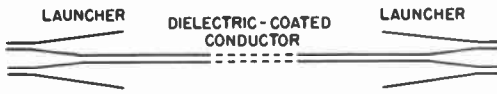
Fig. 36—Surface-wave transmission line with launchers at each end. These form transitions to coaxial line. Courtesy of Electronics.
