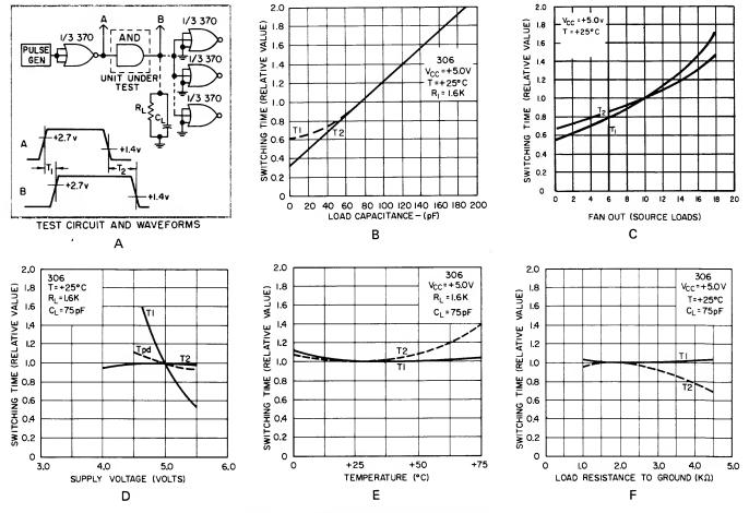
Figure 3 AND Gate Switching Characteristics
