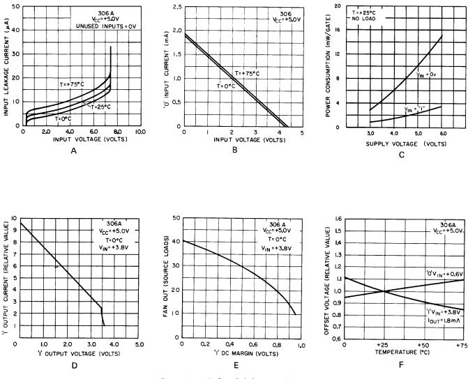
Figure 4 AND Gate DC Characteristics
