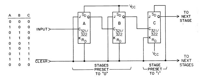
NOTE: Tie all unused J and K inputs to  $V_{\mbox{CC}}.$
