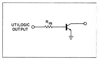
Figure 21 UTILOGIC II to RTL Interface
