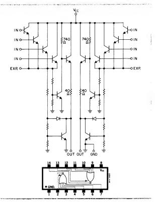
Figure 6 317 Dual 4-Input Expandable NOR Gate
