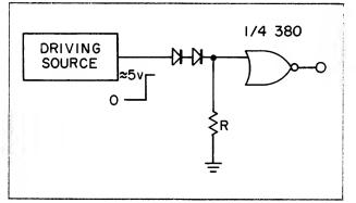
Figure 23 5 Volt to Source Input Interface
