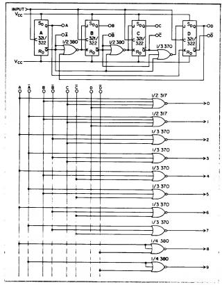
Figure 46 BCD Counter with Decimal Decoding
