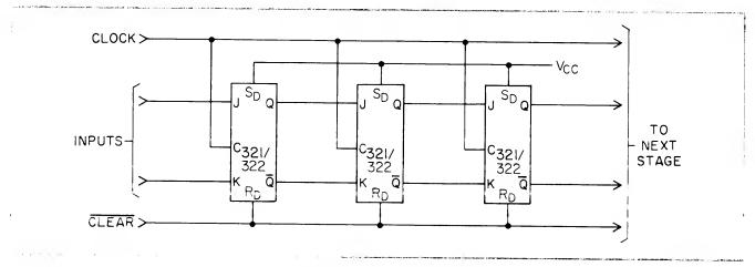
Figure 38 Serial Entry Shift Register
