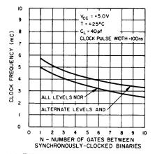
Figure 44 Effect of Logic Depth on Clock Frequency
