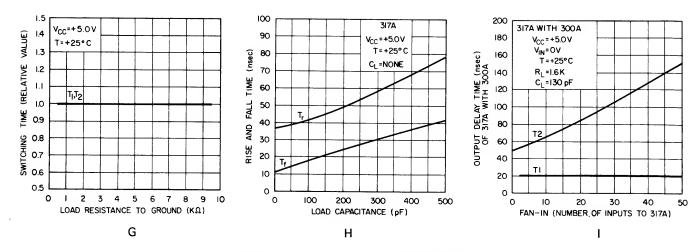
Figure 10 NOR Gate Switching Characteristics
