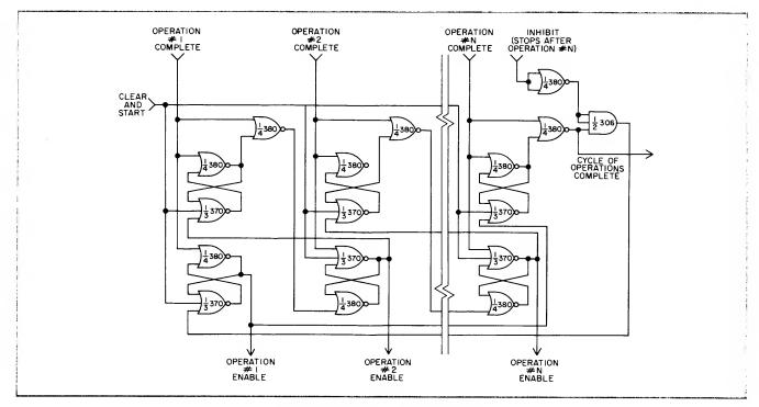
Figure 54 Asynchronous Sequencer
