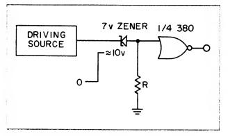
Figure 24 10 Volt to Source Input Interface
