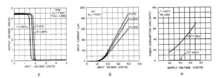
Figure 11 NOR Gate DC Characteristics
