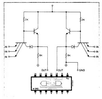
Figure 2 306 Dual 3-Input AND Gate
