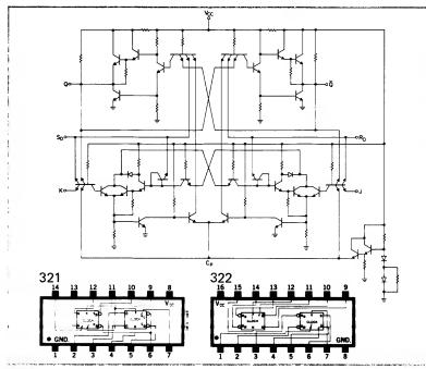
Figure 16 321, 322 Schematic Diagram
