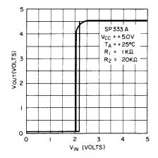
Figure 61 Schmitt Trigger V<sub>IN</sub> vs V<sub>OUT</sub>
