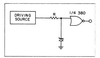
Figure 25 Interfacing with Variable Input Levels
