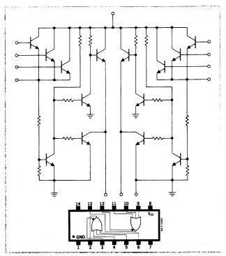
Figure 12 333 Dual 3-Input Expandable OR Gate
