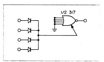
Figure 28 Diode Logic to UTILOGIC II Interface
