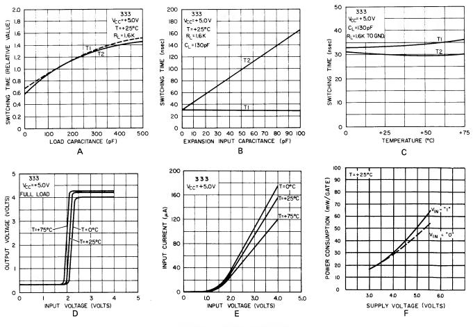
Figure 13 OR Gate Characteristics
