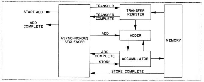
Figure 53 Asynchronous System
