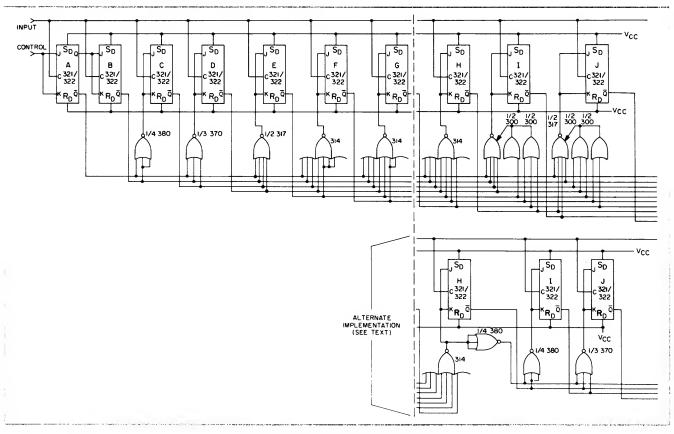
Figure 43 Synchronous Binary Counter
