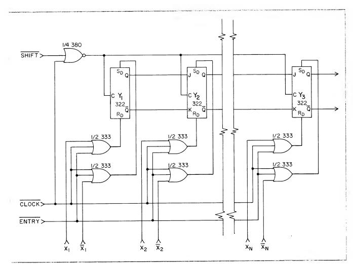
Figure 39 Parallel Entry Shift Register
