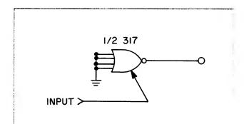
Figure 27 Low Level to UTILOGIC II Interface
