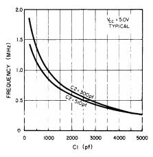
Figure 63 Oscillation Frequency
