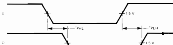
Fig. 2 TURN-ON & TURN-OFF DELAYS DATA TO OUTPUT
