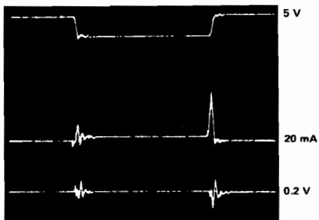
b) SN74S00 load: C_L = 50 \text{ pF}
