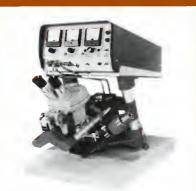
Parallel-gap Welder. New dynamically controlled welder is designed to weld ribbon leads of semiconductor networks to selected printed-circuit materials . . . reducing cost and improving reliability of network-to-PC-board connections.
