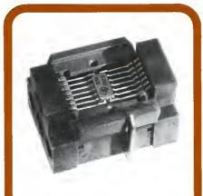
**Test Socket.** SN008 is designed for inspection and engineering breadboarding of networks in Mech-Pak carrier. Also, it is a convenient test fixture. Designed for extended use at 125°C.
