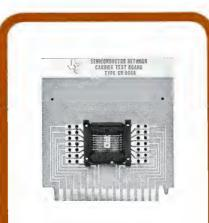
**Test Board.** SN006A is for incoming inspection and engineering breadboarding of networks in Mech-Pak carrier. Designed for extended use at 125°C. Uses Amphenol No. 143-015-01 printed-circuit connector or equivalent.
