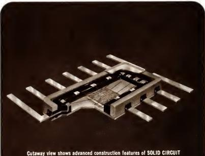
itaway view shows advanced construction features of SOLID CIRCUIT semiconductor networks
