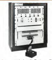
Integrated-circuit Testers. TI offers several types of high-speed automatically sequenced testers for production use. The Model 659A, for example, performs 36 tests in less than 1½ seconds.
