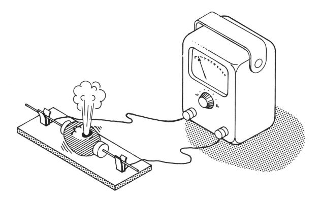
In some instances, an ohmmeter may be used to indicate opens or shorts. Any tester selected should be checked by the user to assure that it does not apply voltages or currents exceeding the ratings of the device being tested.
