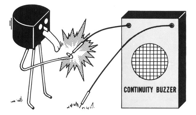
Wiring continuity tests can be made safely by use of a selected ohmmeter or electronic buzzer, that is, one that does not exceed the current or voltage ratings of the devices in the circuits being tested.
