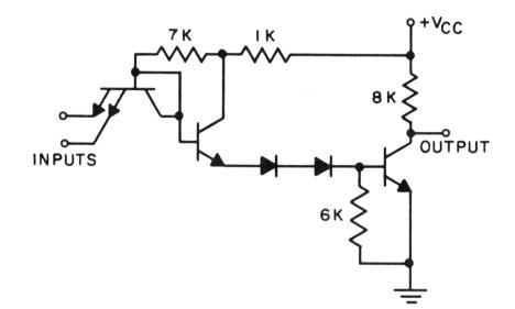
DIGITAL INTEGRATED CIRCUITS DTL (5.0V & 4.5V)
