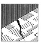
Cracked substrate due to shock
