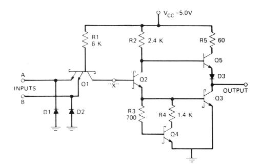
DIGITAL INTEGRATED CIRCUITS TTL(M) 5.0V
