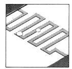
"Pinhole" due to manufacturing defect
