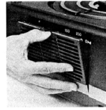
Figure 1. Remove the side cover like this.
