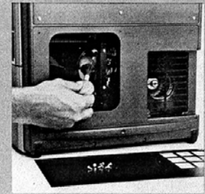
Figure 4. Stand the projector on edge. Remove the air filter and the base plate. This permits all visible parts to be cleaned using a brush and air blower.
