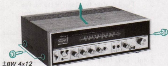
Fig. 2-1. Wooden case removal
