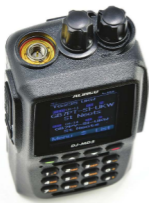
The SMA aerial connector accompanies the channel and volume controls on the top panel.
