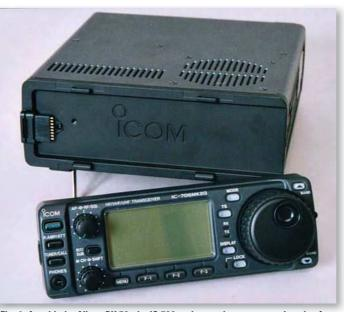
Fig. 4: As with the Alinco DX-70, the IC-706 series can have a remote location for the control head, making it easier to remove the unit, when not in use.
