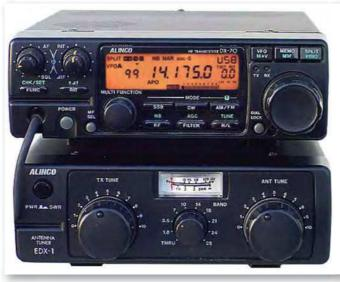
appeared in early 1995, and offers h.f. and 50MHz transceiver coverage on amplitude modulation (a.m.), c.w., narrow band frequency modulation (n.b.f.m.) and s.s.b. The rig
