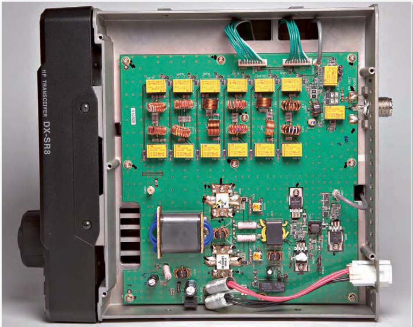
The single-board r.f. power amplifier stage and relay-switched band filters.
