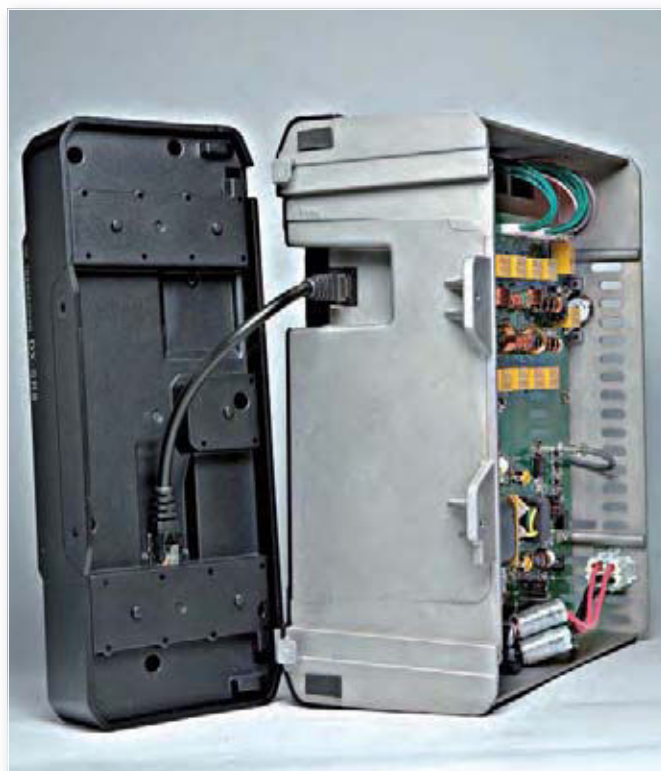
The whole front-panel pivots off for remote operations after releasing two screws – various length leads are available as extras.
