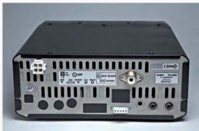
The simple back panel has little more than sockets for the power, antenna, accessories, Morse key and external speaker along with a coaxial socket to add in an external ALC voltage.
