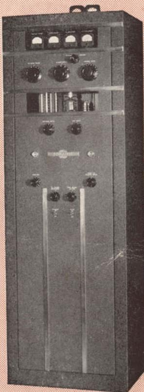
The 310A Exciter Unit (for the 30K). Single Dial Tuning. Permeability Tuned Oscillator Control. Bandswitching.
