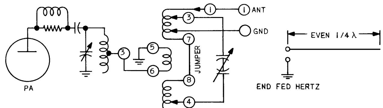
Figure 3-2 Typical Antenna Tuner Circuits
