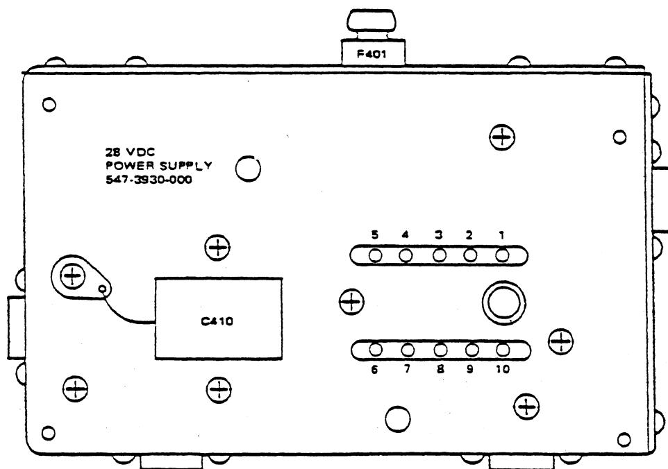
28-Vdc Power Supply, Bottom View, Terminal Location
