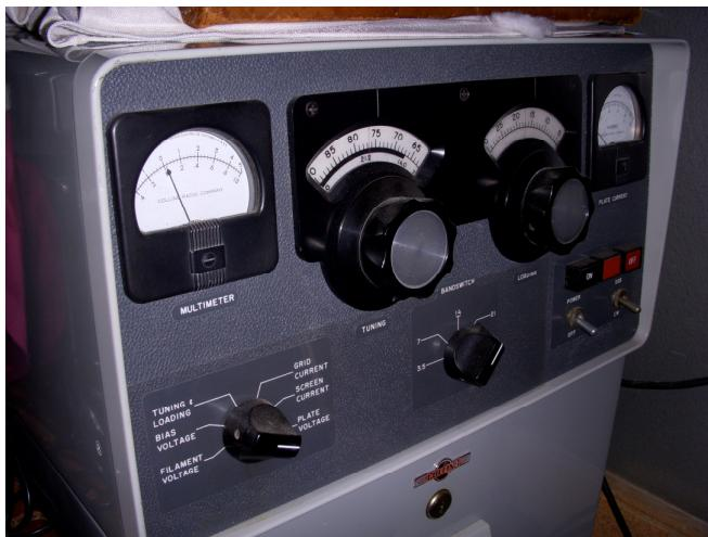
There is one last tidbit of confusion that I see about tuning. Without going into a lot of technical detail, the Tuning knob sets the resonant frequency of the tuned circuit in the output of the PA. Setting this circuit to resonance allows maximum transfer of power from the amplifier to the load - for a given loading condition. The tube in your 30S-1 has two different Current vs. Voltage (I-V) characteristics. The first
