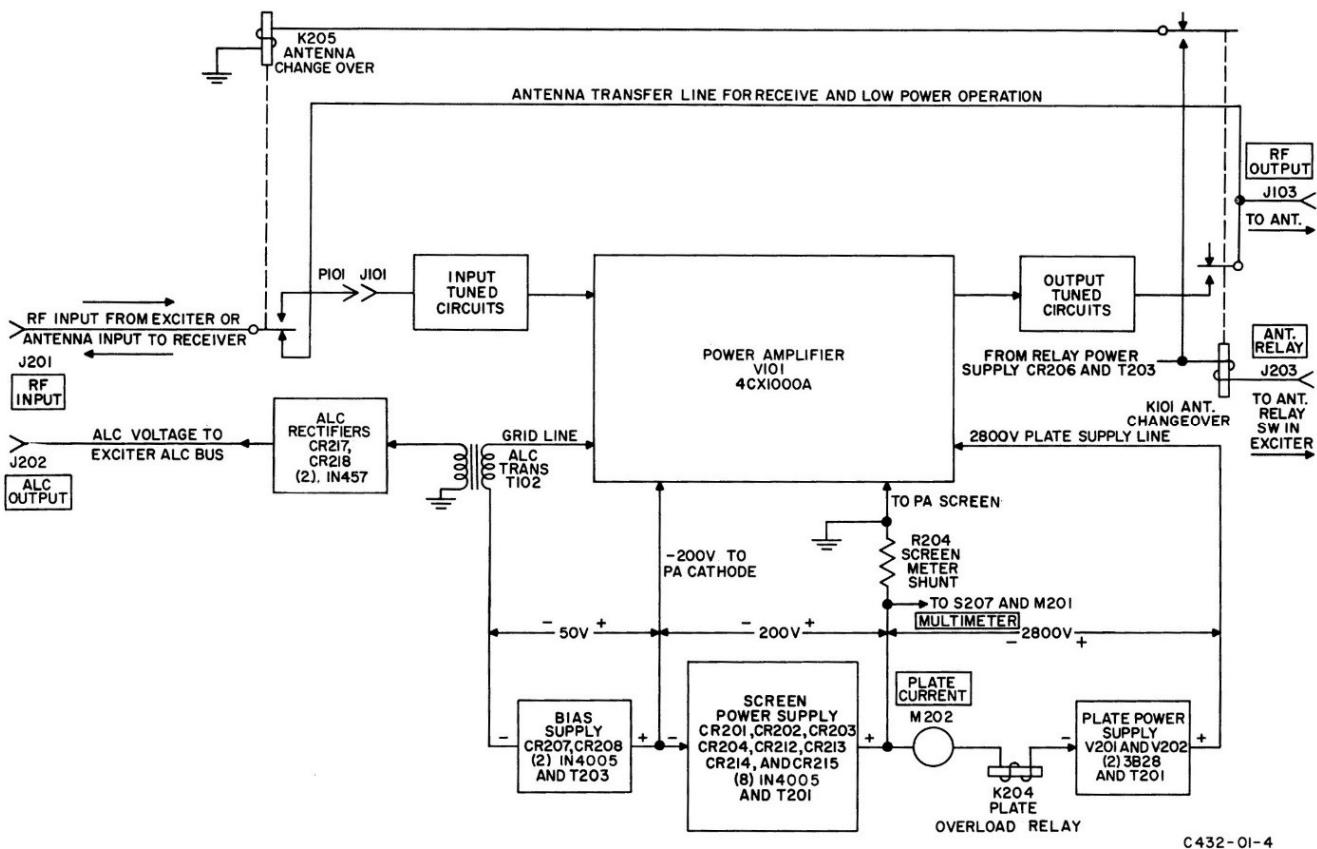
instantaneous Screen Grid voltage is now north of 390 (RF + DC) volts peak (you pick your poison) and the tube is getting right up there against the screen limit. There is no margin there for error.
