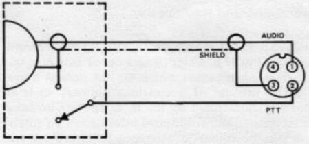
Figure 2-3. TR-7 Microphone Connection
