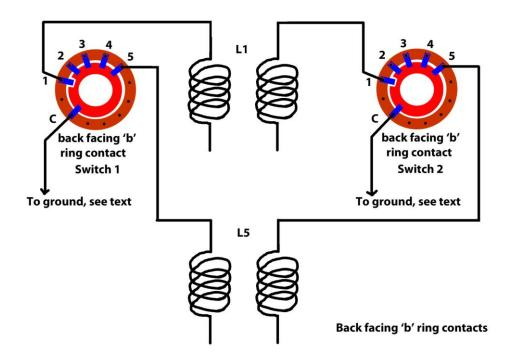
Note that the common terminal 'C' for the 'f' and the 'b' sides of the switch are **not** the same terminal, they are separated by one index position.
