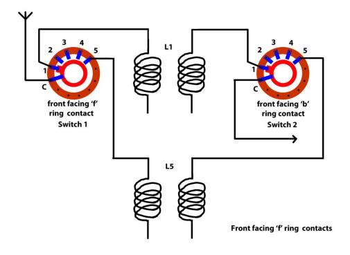
Note that in each section the highest frequency's coils are positioned nearest to the wafer switch.
