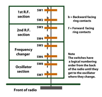
The front facing contacts select the required coil, the back facing contacts de-select that coil from being grounded.
