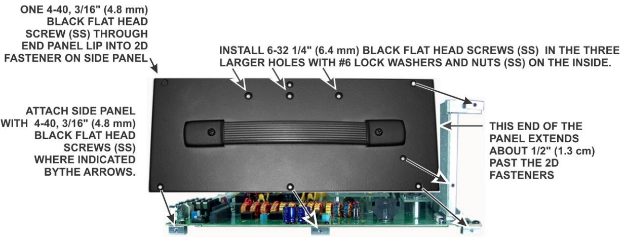
Figure 65. Mounting Left Side Panel.
