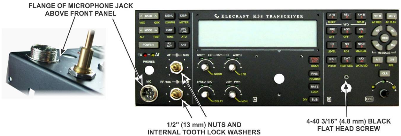
Figure 11. Mounting the Front Panel on the Front Panel Board.
