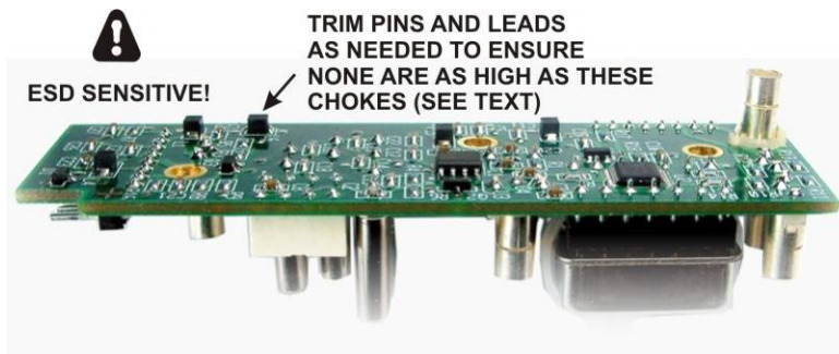
Figure 77. Checking Lead Lengths on KREF3 Board.
