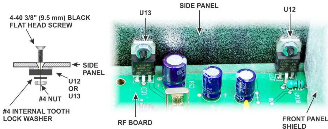
Figure 74. Attaching U12 and U13 to the Right Side Panel.
