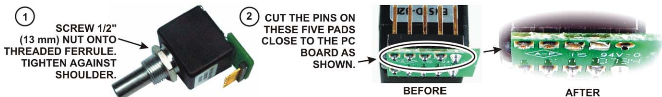
Figure 14. VFO B Encoder Assembly Preparation for Installation.
