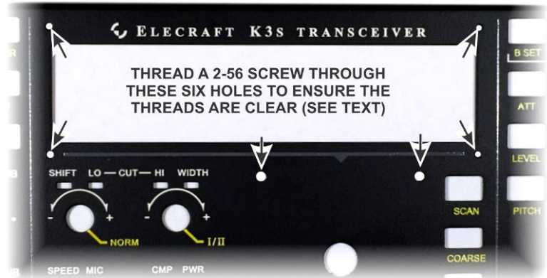
Figure 10. Checking Front Panel 2-56 Threaded Screw Holes.
