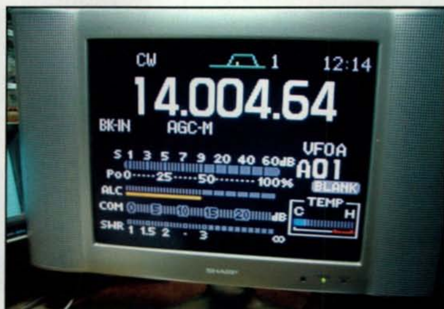
Photo 5— Normal display on remote 13-inch LCD monitor. An expanded font may also be selected.
