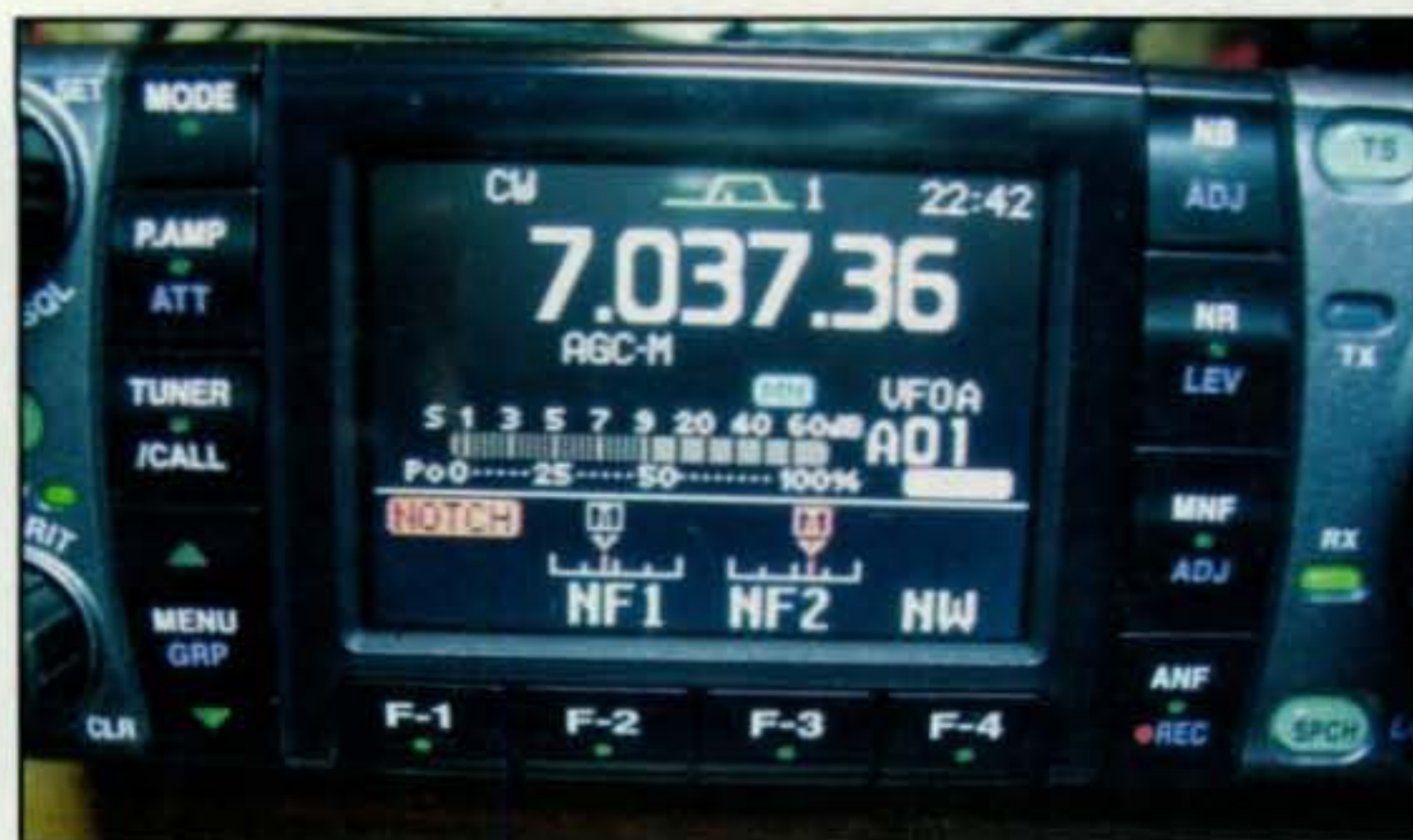
Photo 8— The two manual notches are easy to set. Here NF1 is just below, and NF2 is just above center.
