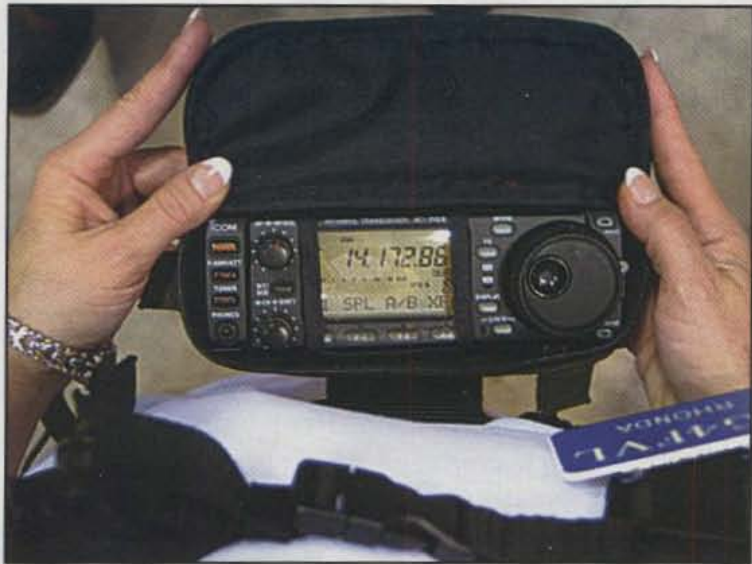
Photo 4— Rhonda shows us the IC-703's front panel/controller, which is carried in its belt clip pouch and connected to the transceiver's main body by an optional OPC-581 controller/rig separation cable.
