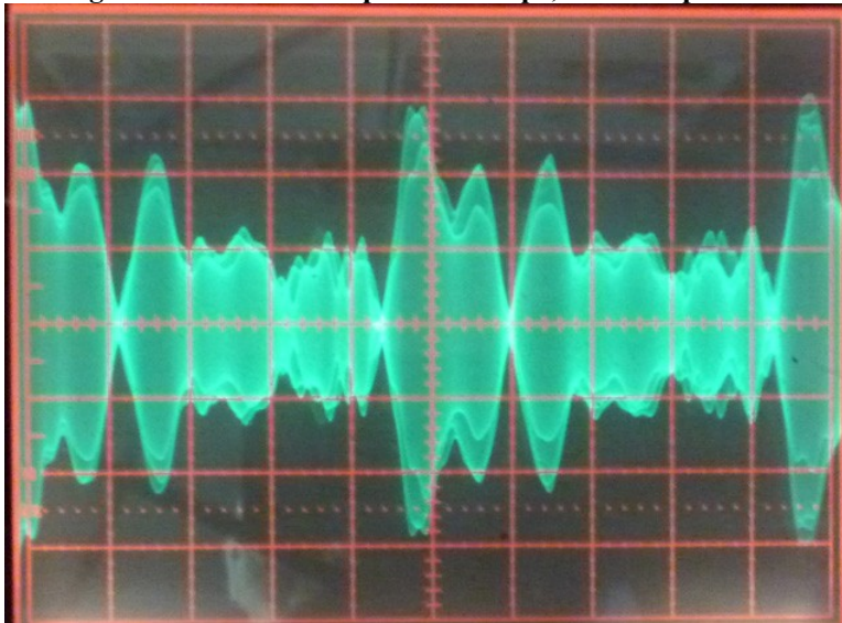
Figure 17: 100W PEP speech envelope, 6 dB compression.
