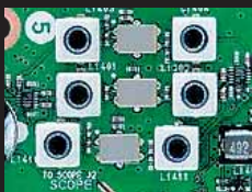
Three roofing filters
