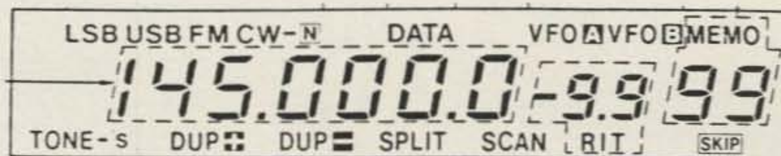
Fig. 2—Overview of the IC-275's main display indicates readout of frequency memory, VFO, mode, scan, etc.
