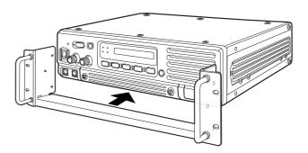
(3) Tighten the supplied screws (M4  $\times$  8) and the 2 screws removed in step (1) to each side. (6 screws in total)
