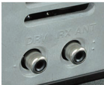
Figure 5-2 DRV and RX ANT Connectors
