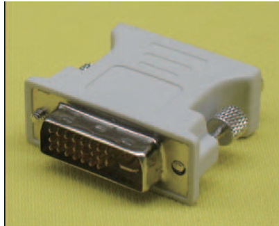
Fig. 77 DVI (Male) - VGA (Female) Conversion Connector (Example)
