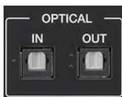
Fig. 138 OPTICAL IN and OPTICAL OUT Terminals
