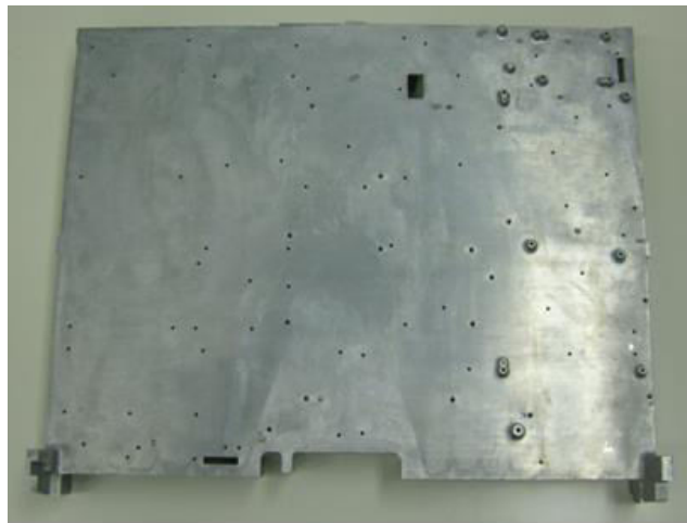
Fig. 5 Chassis (Upper Surface)
