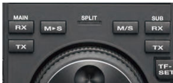
Fig. 101 Key Allocation Suitable for Split Operation
