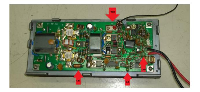
If you still have a short or low resistance across along the main bus/power leads after testing all of the transistors in the PA, then you will have to perform what I refer to as a "board sweep". I start at one end, usually near the power leads, and test each resistor and capacitor for a fault. Test electrolytic capacitors C24, C18, and C12 first. I've never actually seen a shorted capacitor in a 930S PA, but anything is possible. This is a tedious, last-ditch process.
