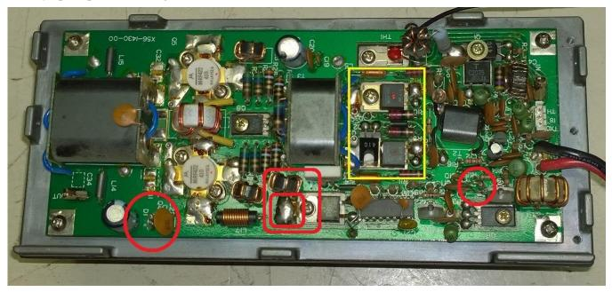
The famous "Red Dot" Motorola MRF485 driver transistors that you've probably heard about are boxed in yellow. The red dot denotes low current gain, also known as Beta or hFe. These have not been manufactured for years, as they were a special "run" for these radios by Motorola. I'll explain the red circles and squares on the following pages. Schematically, the 930S "Final Unit" has a 28 volt power bus running right down the middle, marked in red.
