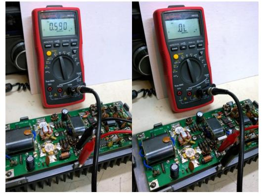
If you get something other than what you see, especially a reverse voltage (or a low resistance) then you have one or more bad drivers. I've NEVER seen a driver with just a bad Base-Emitter or Base-Collector junction. The Collector-Emitter is also bad – it either shows a low resistance in each direction, or it's completely open. Sometimes Q2 is open, while Q3 is good in the forward direction with leakage in the reverse.
