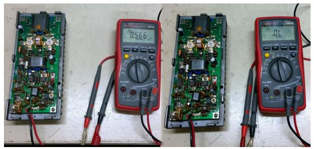
MY READINGS FOR OPTIONS 2 AND 4: Here are the test readings from my Options 2 & 4 power amps.
