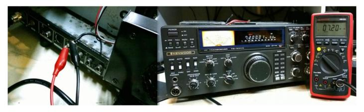
The same test is shown below, but using R174 with my rig set at 14.200 MHz. I've connected a scope probe here, but a J-hook works too. To use the resistor, you will have to scrape some paint from the wire lead shown above (arrow).
