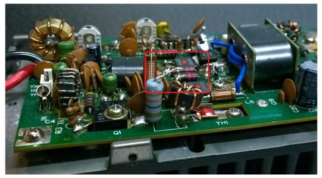
Now repeat 4a and 4b. If Q1 tests good, the problem must be either in the Final Output stage (Q4 & Q5), or the CONTROL circuitry. Reconnect L3 before putting your PA back in service.
