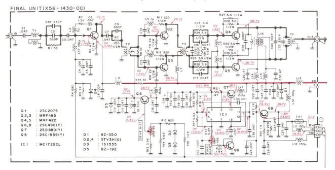
Kenwood conveniently arranged the schematic so that the SIGNAL amplification circuitry consisting of Q1, Q2 + Q3, and Q4 + Q5 and their associated components are located above the bus line, and the CONTROL circuitry consisting of Q6, Q7, Q8, Q9, and IC1 are below the bus line. However, it's NOT always arranged that way on the PA circuit board. I list Q2 + Q3 and Q4 + Q5 as pairs because they are arranged in a push-pull configuration.
