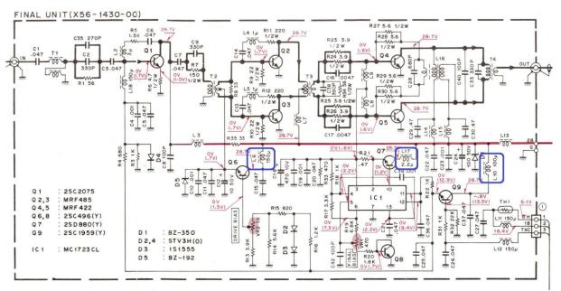
The chokes are L6, L17, and L10. The only control circuit part that I've ever found to be bad while repairing PA's was Q9: A 2SC1959(Y). It was shorted, which dragged down the bus. Q9 is located right next to the PA main power leads. If you look at the schematic you will see that the base and collector of Q8 are shorted together, which essentially turns this transistor into a diode. TH1 is referenced in the Signal Unit control circuit tests in the Appendix.
