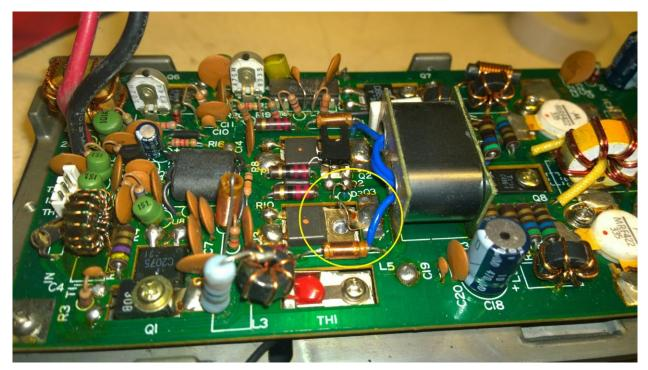
**IMPORTANT:** Even with the drivers removed, your PA should pass tests 1a and 1b, but with a higher forward voltage - around 0.630. The reverse will be still be zero, or OL. The reason for the higher forward voltage is that you will have one less pair of C-E junctions in the mix. If you remove your drivers, and this test shows a low resistance in either direction, or the same reading each way, then you have a problem elsewhere in the PA. You MUST find out why BEFORE you install new drivers.
