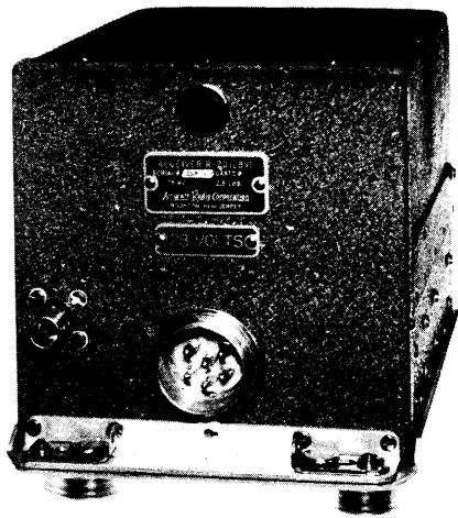
Type R-20 Receiver (75 mc) Shown with M-23 Mounting
