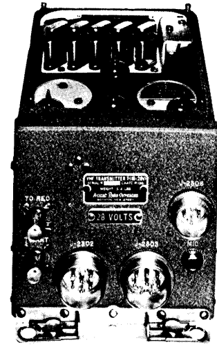
ARC-16950 Ten Channel Adapter shown installed in Type T-11B Transmitter
