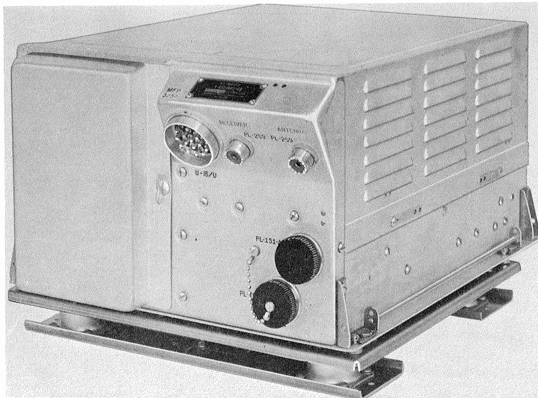
Figure 1-8. Radio Transmitter T-452/ARC-49 on Mounting Base MT-238C/ARC-3
