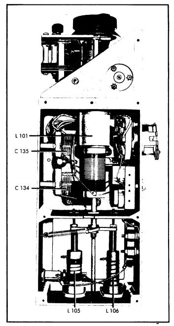
Figure 5-8. High Frequency Oscillator
