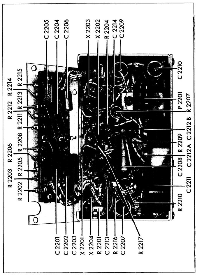
Figure 8-9. MCW-CFI Unit --- Bottom View
