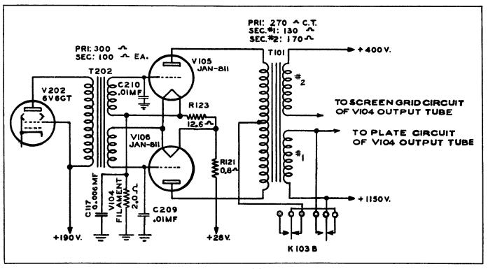
Figure 4-7. Modulator Circuit
