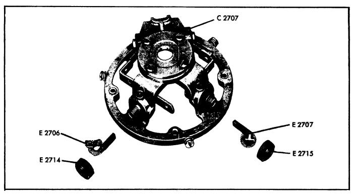
Brush Housing Assembly for 400-Volt Commutator
