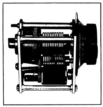
Figure 4-15. Singleturn Autotune Unit (Type 96J)— Left Side View
