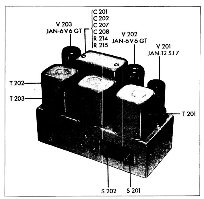
Figure 8-10. Audio Amplifier Unit --- Top View
