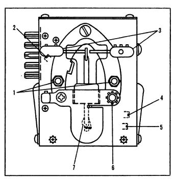
Figure 5-11. Keying Relay K102 and Vacuum Contact \$116
