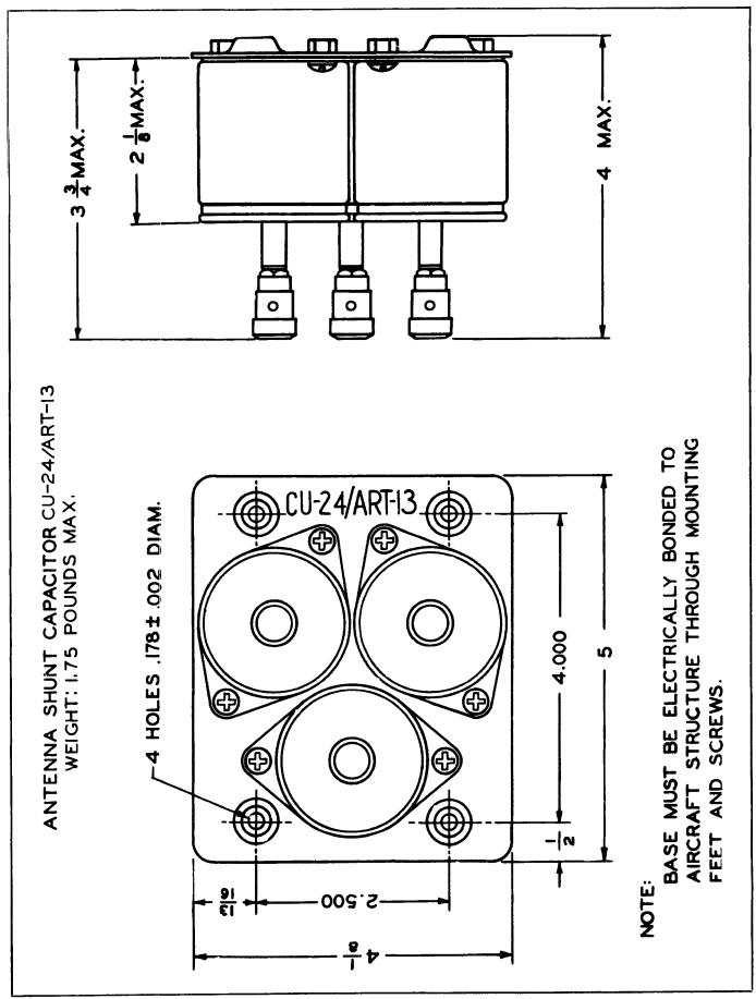
Figure 8-29. Antenna Shunt Capacitor CU-24/ART-13 — Outline Dimensions
