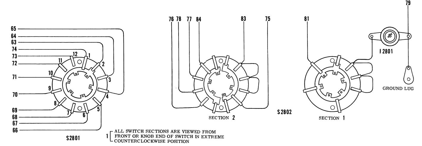
Figure 8-40. Control Panel C-405/A — Practical Wiring Diagram
