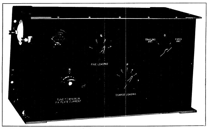
Figure 8-21. Antenna Loading Unit CU-32/ART-13A — Front View
