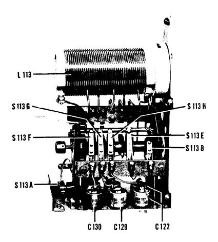
Figure 8-15. Multi-Element Switch — Right Side View
