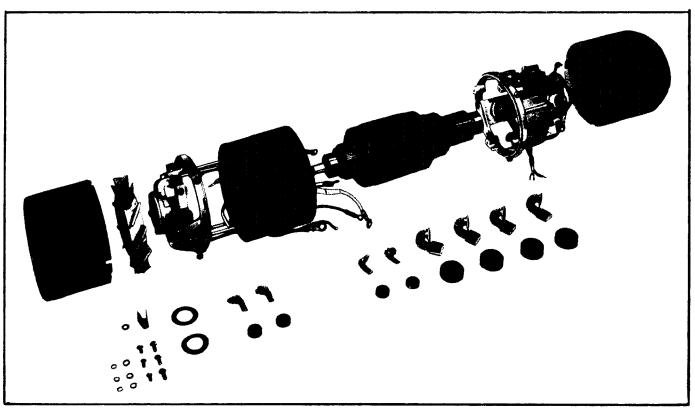
Figure 5-4. Component Parts of Russell Dynamotor
