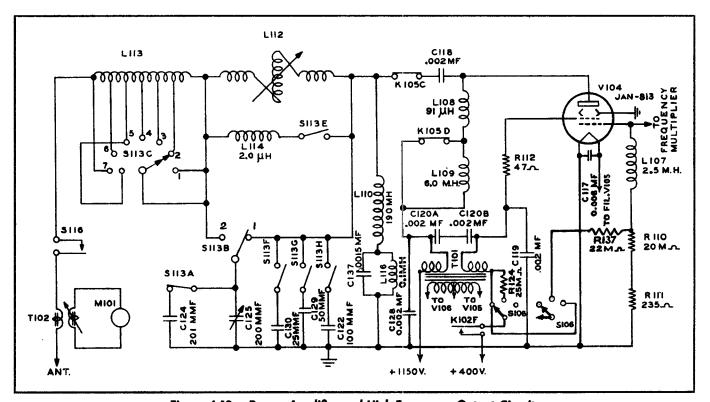
Figure 4-13. Power Amplifier and High Frequency Output Circuits
