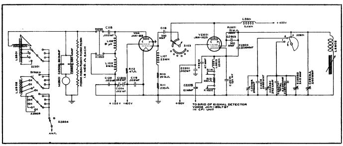
Figure 4-11. Low Frequency R-F Circuits
