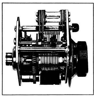
Figure 4-17. Multiturn Autotune Unit (Type 96K)— Left Side View
