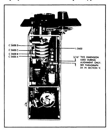
Figure 5-7. Low Frequency Oscillator
