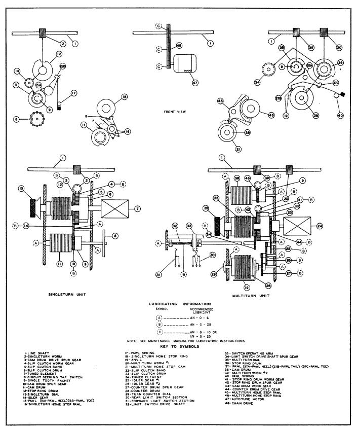
Figure 4-14. Autotune Mechanism — Mechanical Portion
