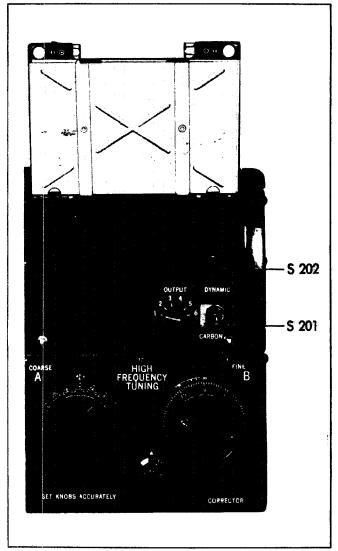
Figure 2-2. Microphone Selector Switch and Sidetone Output Switch
