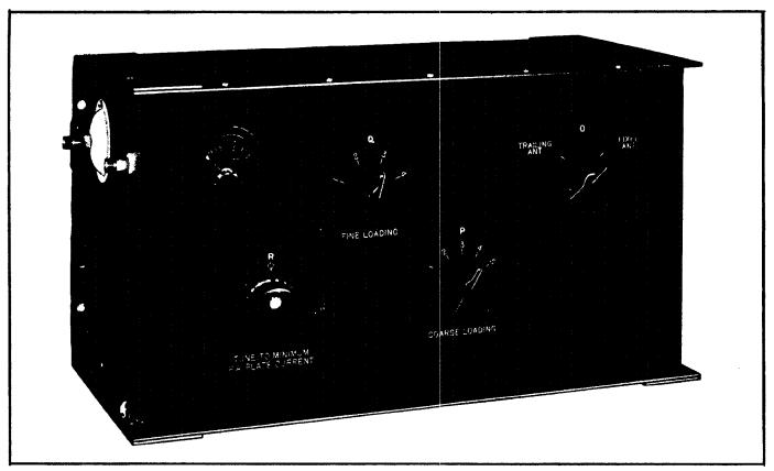
Figure 1-7. Antenna Loading Unit CU-32/ART-13A—Front View
