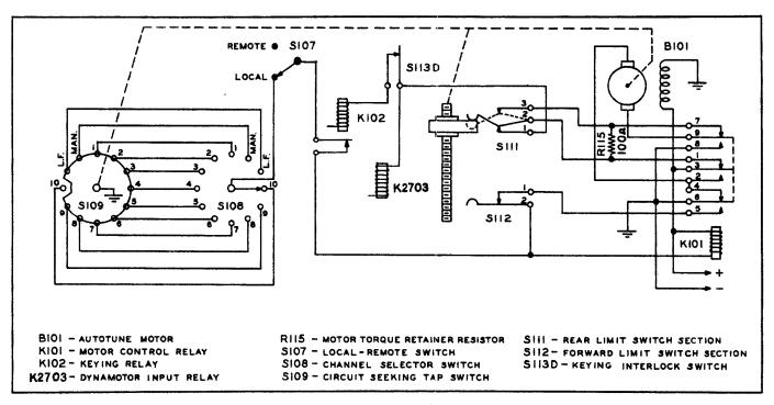
Figure 4-20. Electrical Portion of Autotune System
