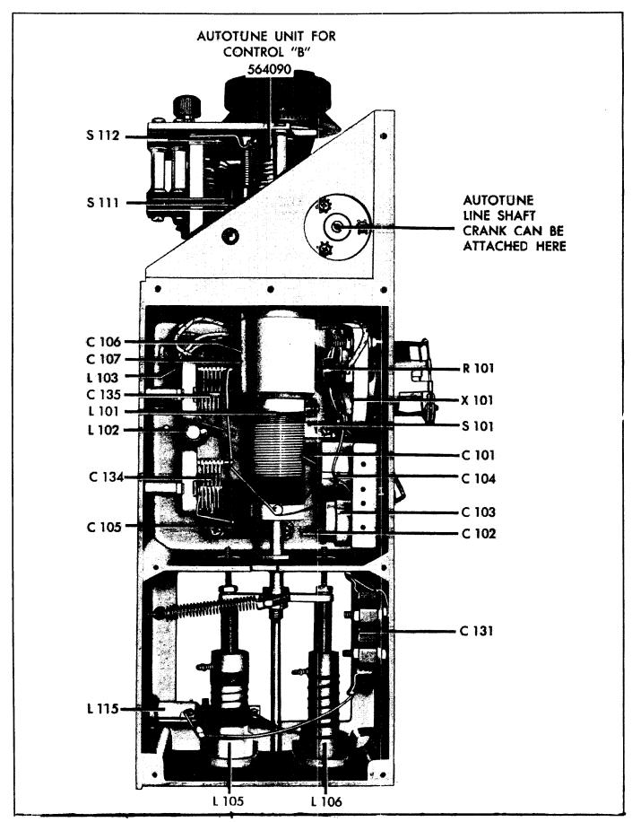
Figure 8-6. High Frequency Oscillator — Side View, Open
