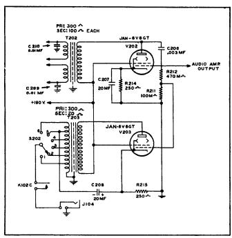
Figure 4-8. Sidetone Amplifier Circuit
