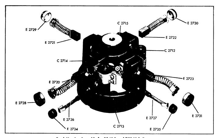
Brush Housing Assembly for 28-Volt and 750-Volt Commutators
