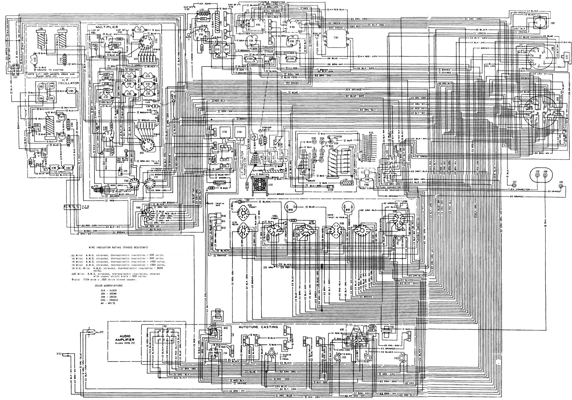
Figure 8-41. Radio Transmitter T-47A/ART-13 — Practical Wiring Diagram
