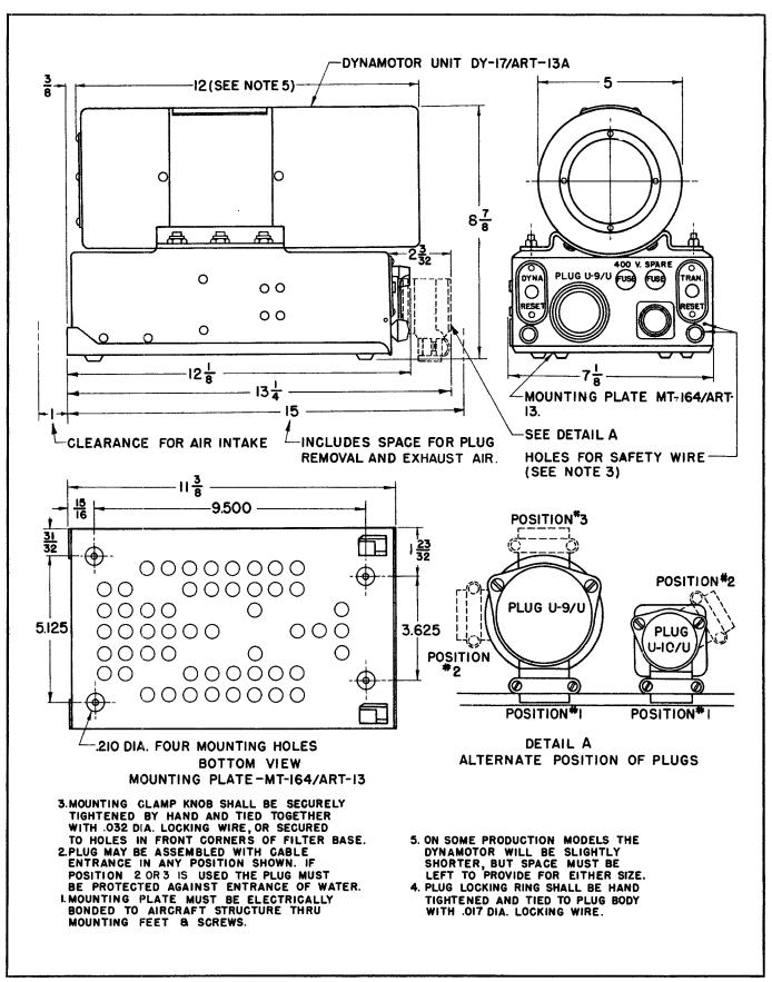
Figure 8-31. Dynamotor Unit DY-17/ART-13A — Outline Dimensions
