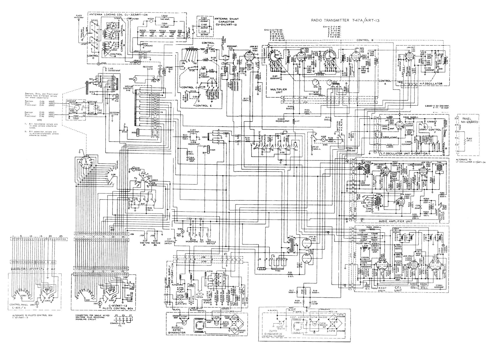
Figure 8-42. Radio Transmitting Set AN/ART-13A — Schematic Diagram
