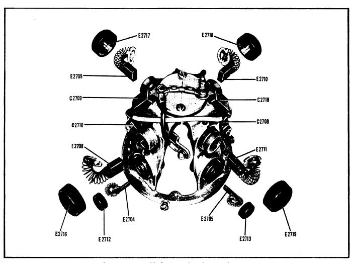
Brush Housing Assembly for 28-Volt and 750-Volt Commutators
