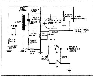
Figure 4-9. MCW Oscillator Circuit
