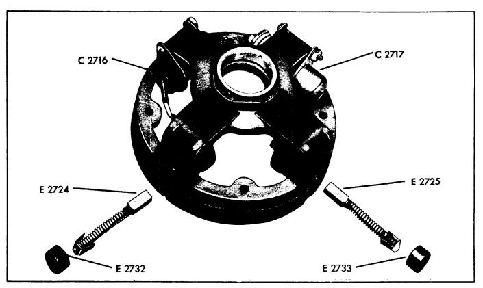
**Brush Housing Assembly for 400-Volt Commutator**
