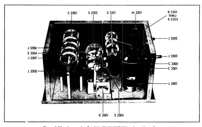
Figure 8-22. Antenna Loading Unit CU-32/ART-13A — Rear View, Open
