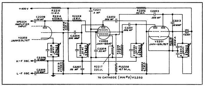
Figure 4-10. CFI Oscillator Circuits
