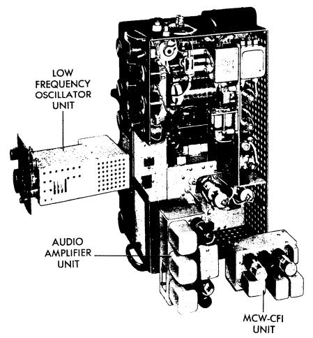
Figure 5-6. Radio Transmitter T-47A/ART-13 and Removable Units
