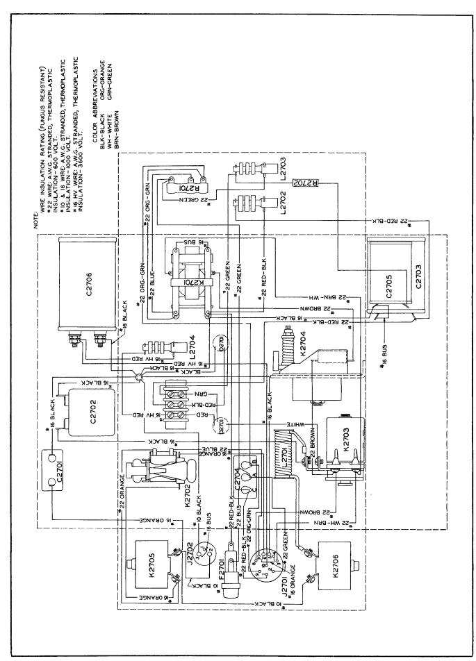
Figure 8-39. Dynamotor Unit DY-17/ART-13A — Practical Wiring Diagram
