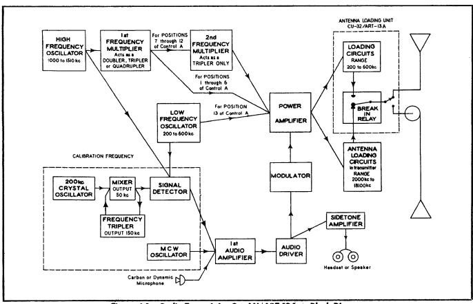
Figure 4-1. Radio Transmitting Set AN/ART-13A — Block Diagram
