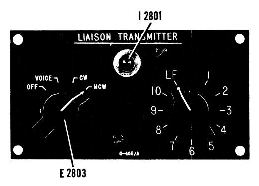
Figure 8-19. Control Panel C-405/A — Front View
