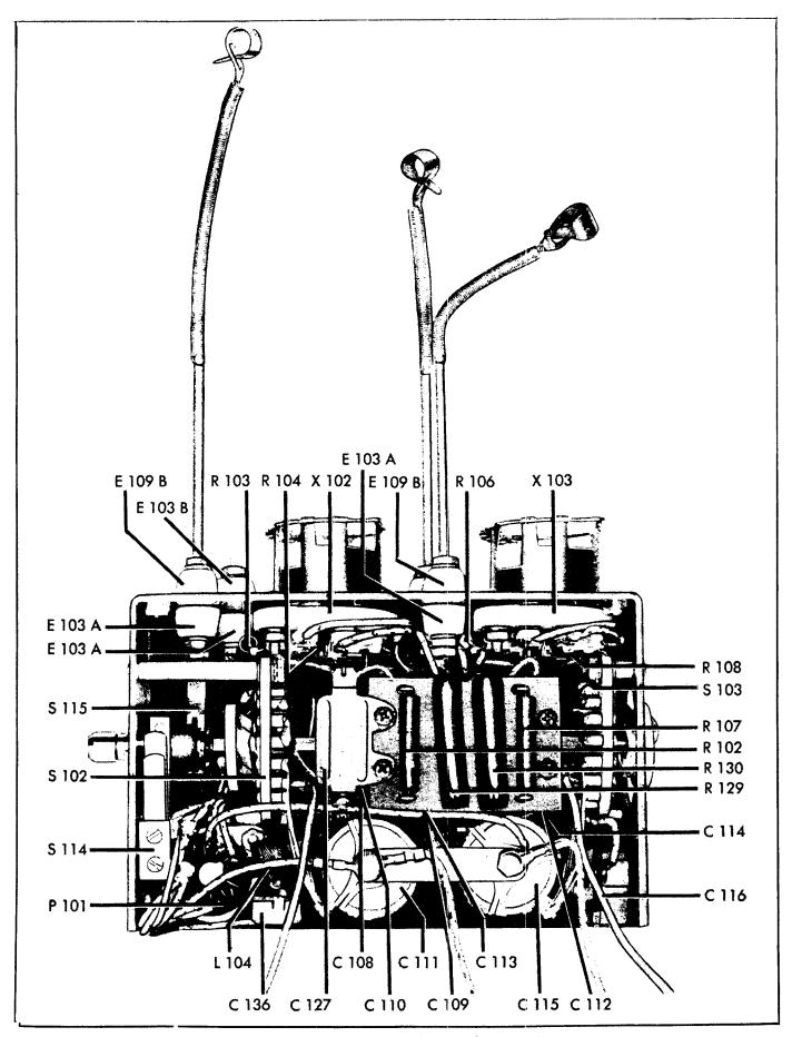
Figure 8-7. Frequency Multiplier -- Side View, Open
