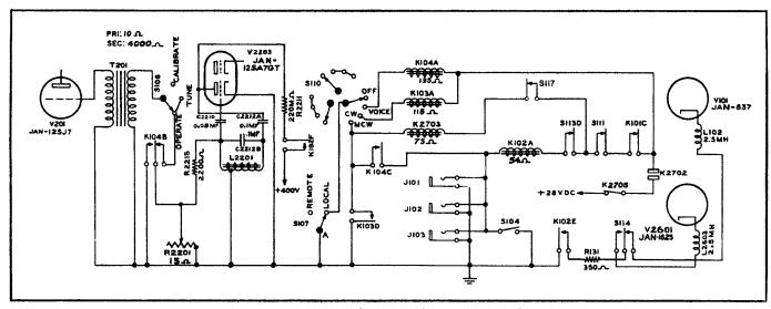
Figure 4-5. Emission Selection and Carrier Control Circuits
