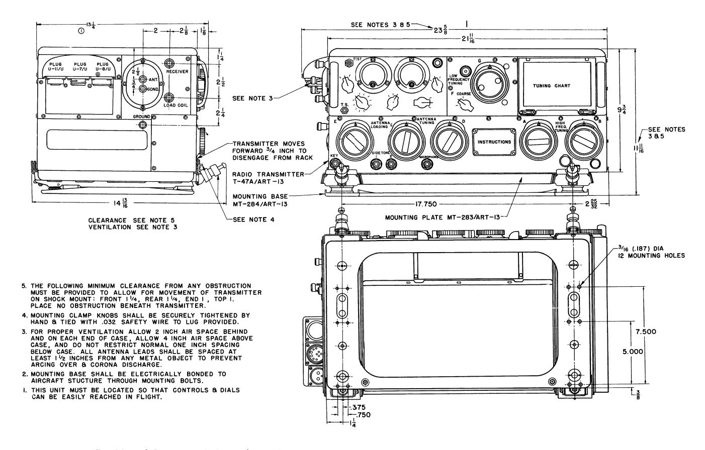
Figure 8-25. Radio Transmitter T-47A/ART-13 — Outline Dimensions
