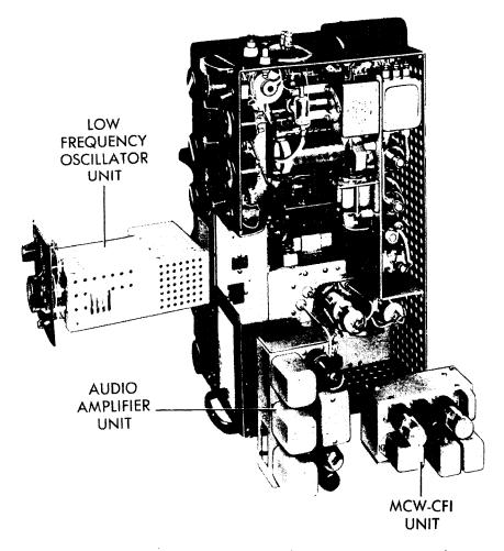
Figure 1-3. Radio Transmitter T-47A/ART-13 — Units Removed
