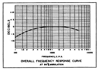
Figure 6-1. Overall Audio Frequency Response Curve
