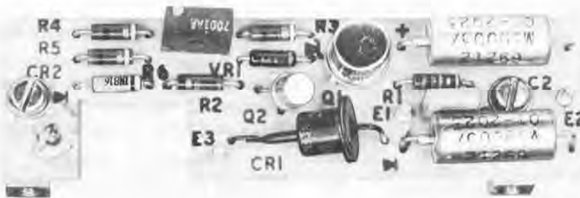
Figure 3-8. Terminal board 1A1A2A8A2, parts location diagram.
